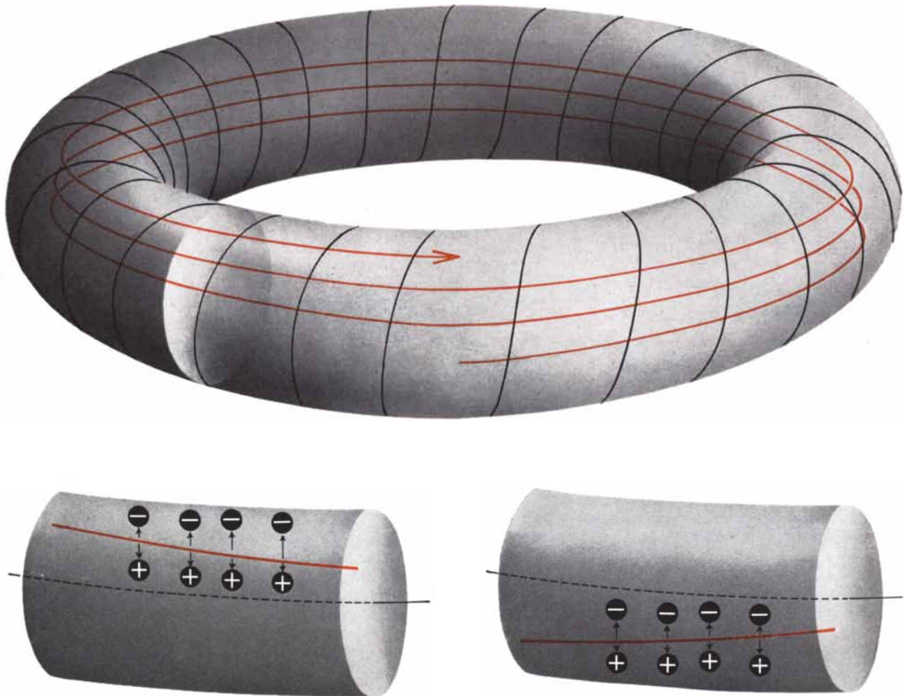
TWISTED MAGNETIC FIELD counteracts tendency of charges to separate. Top diagram shows a part of one line of force, which, if drawn for its whole length, generates a ring-shaped surface. Each
