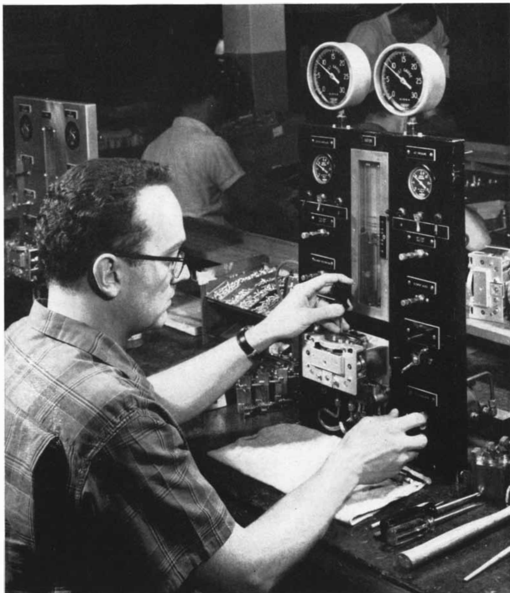
Test-panel calibration of the Foxboro Consotrol Controller. Its exclusive floating-disc design has introduced new simplicity and dependability in process control systems.
