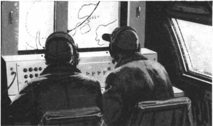
AIR CONTROL relays commands from ground station to drone where distance or terrain block direct beam. Air director may also originate control since it has complete microwave system.
