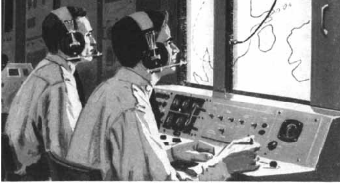
GROUND CONTROL of target drone centers in air-portable van. Men at console maintain control through flight instruments. Path of drone is traced automatically on plotting board at right.
