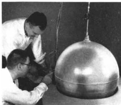
Figure 1—Testing a Tapco-made forged-and-welded titanium pressure vessel under actual operating conditions at 5,000 psi and -320^{\circ}\text{F} .
