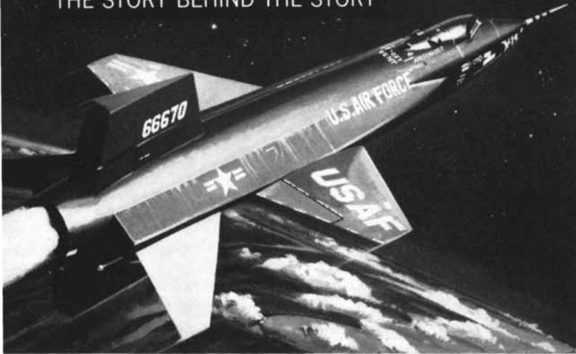
HYPERSONIC X-15 , powered by a mighty rocket engine, will follow bullet-like trajectory during flight, similar to path of ballistic missile.
