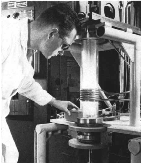
This Hughes engineer, shown growing a silicon ingot, is part of the team of engineers and scientists who are continually probing the frontiers of advanced electronics.
