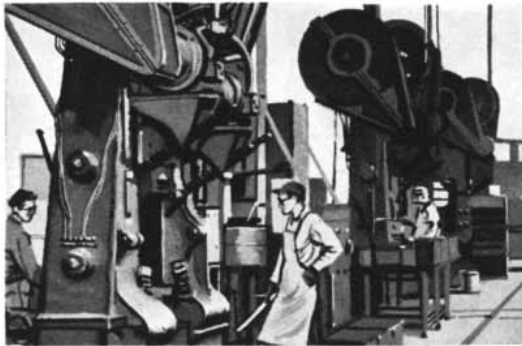
Bearings on drop hammers in Curtiss-Wright's forging shop failed after ten months. Mobil recommended a grease that extended bearing life five years . . . saved $1,152 every ten months.
