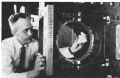
Optical purity and a high softening point (1585° C.) make Corning's 100% Fused Silica useful in wind tunnel windows.
