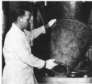
Exit cones capable of withstanding temperatures of 6000° F, represent one example of advanced engineering being performed by the Hughes Plastics Laboratory.
