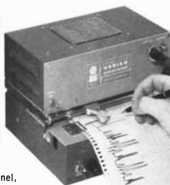
Varian G-10 bench-top recorder for accessible, horizontal chart.
