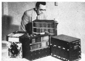
The completely transistorized RW-30 airborne digital computer has a volume of 4.19 cu. ft. and weighs only 203 lbs., including power supply
