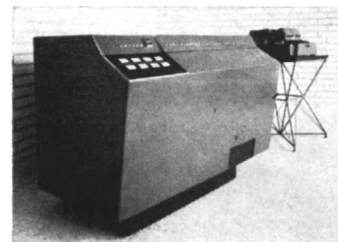
The RW-300 digital control computer has broad applications in automatic process control, data reduction and test facility operation
