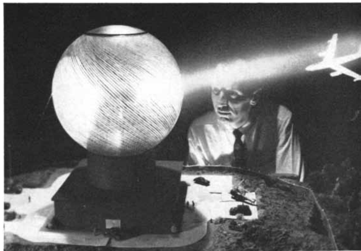
NON-ROTATING 360° RADAR ANTENNA. Only the feed point moves. Principle involved will permit economical construction of very large high gain scanning antennas. Application of inflation techniques will permit lighter-weight long-range air-transportable radar. Working models already built and evaluated. Electronics Division and Research Laboratories
