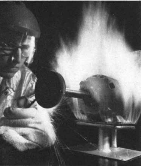
HIGH TEMPERATURE ELECTRICAL INSULATION. Effective for long periods at 500° C—eventual applications to 1000° C now contemplated. Demonstration motor shown above is running red hot. Aircraft Equipment Department, Materials Engineering Departments, and Research Laboratories
