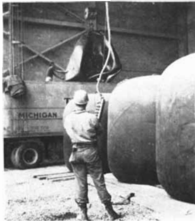
Raw Material —Zirconium tetrachloride is delivered to Mallory-Sharon's sponge plant in 6-ton rubber containers.
