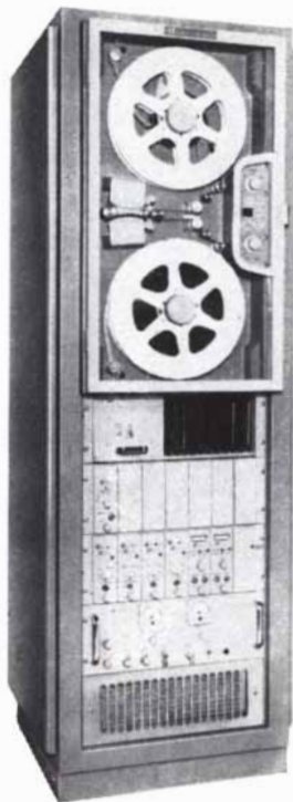
One of three Honeywell magnetic tape systems used to record satellite signals, for pinpoint Doppler analyses of orbits.
