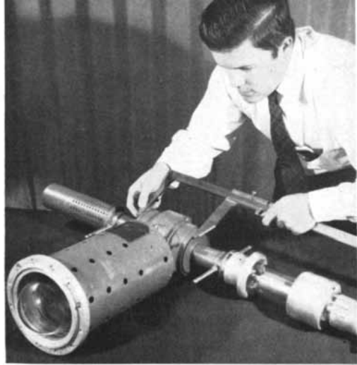
BIGGEST RADAR TUBE. Heart of the longest range shipborne radar ever put in service, a magnetron tube nicknamed "Big Maggie" was developed at the Westinghouse Electronic Tube Plant at Elmira. "Big Maggie" delivers over 10 million watts of peak power, enough to search out enemy planes over 400 miles away.
