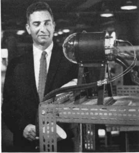
INFRA-RED. Westinghouse has been actively at work in infra-red research, design and development since World War II. Extensive programs are now being conducted for applications of infra-red techniques to present and future military requirements as well as the space age. Pictured is an infra-red seeker, newly designed at Westinghouse Air Arm Division .
