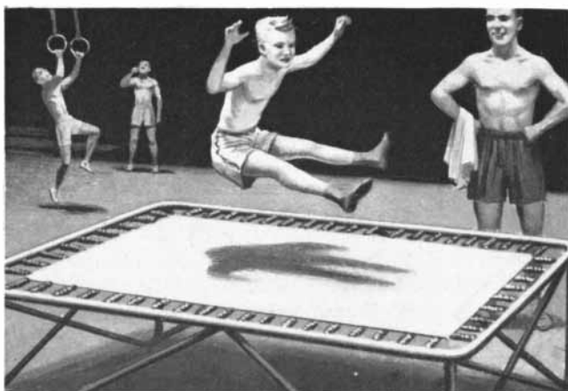
PAPER TRAMPOLINE dramatizes great strength of the new synthetic-fiber papers. Tear strength is about 10 times as great as for a good kraft paper and is actually of the same order of magnitude as woven fabrics. Fold endurance ranges as high as 75 times that of cellululosic papers. The new papers made of nylon, "Dacron" or "Orlon" fibers resist heat, chemicals, weathering, moisture—are dimensionally stable. Potential uses for these new papers are so broad that they are being classed as entirely new engineering materials. We welcome your inquiry.
