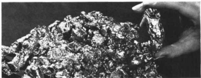
Zirconium Chunklets produced at Ashtabula, Ohio, plant are used to produce ingots for forging or rolling.
