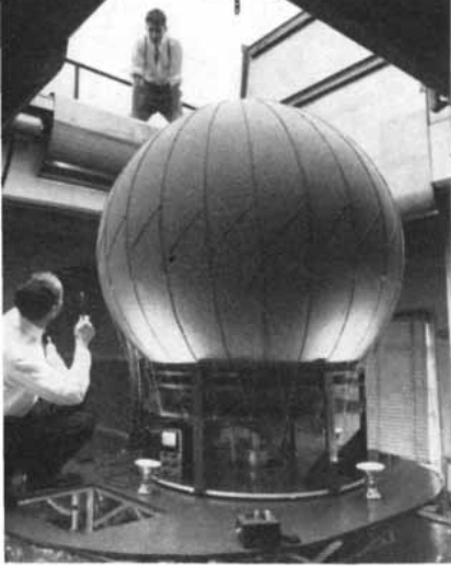
NON-ROTATING ANTENNA. A new kind of radar antenna, the Helisphere is considered a possible forerunner of those to be used for powerful antimissile radars of the future. The antenna, pictured at the Westinghouse Research Laboratories , produces a rotating radar beam without rotation of the antenna structure itself.
