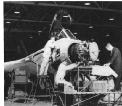
200-MAN FLIGHT TEST FACILITY. Engineers at Air Arm Division install Aero 13-F radar and computer, latest and most advanced radar built by Westinghouse. Flight test facility includes over 200 people and all facilities necessary to completely service, instrument and test avionic equipment in Westinghouse owned and bailed aircraft.
