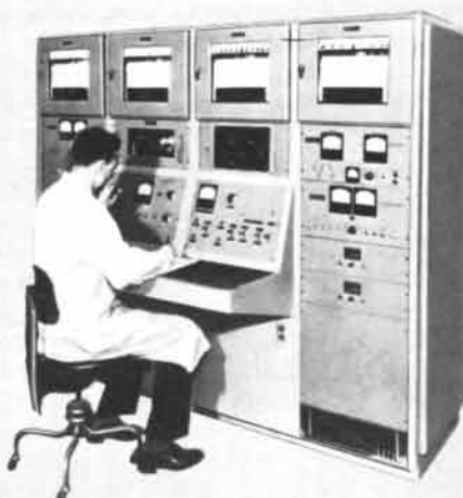
NUCLEAR REACTOR SIMULATOR teams up with Thermal Plant Simulator to provide realistic nuclear power plant training.
