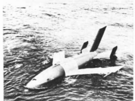
RYAN FIREBEE, with 75% of its exterior surface magnesium, has withstood repeated dunkings in the ocean with no adverse effects. The reason—Ryan applied the proper protective measures.
