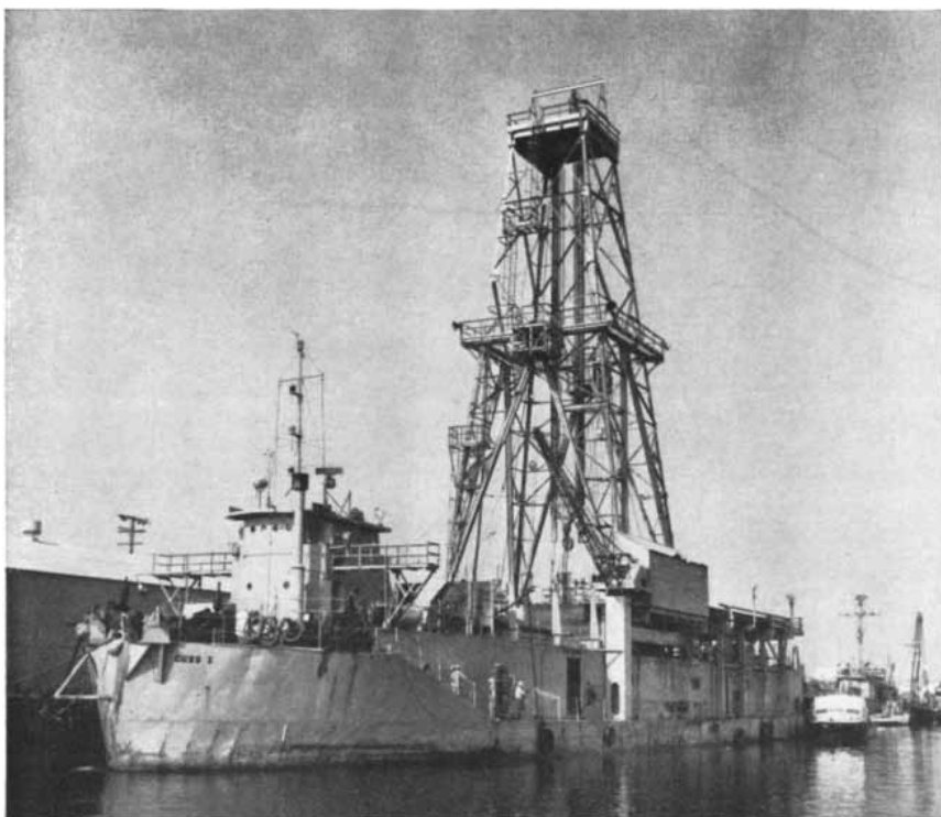
"CUSS I" (left) is an experimental vessel which has been used to drill holes in the bottom off the California coast. The vessel, which is a converted Navy freight barge, is 260 feet
