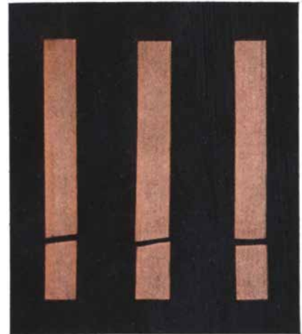
THREE SPRINGS of regular Phosphor Bronze, 5% (A), actual size, took a permanent set at about 200,000 deflections and fractured at an average of 453,374 deflections.
