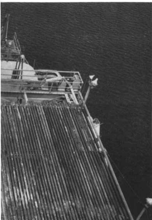
drill pipe can be automatically racked during a single round trip to the bottom.
