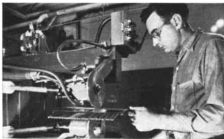
Resistance welding technique on a Budd-designed welding machine.
