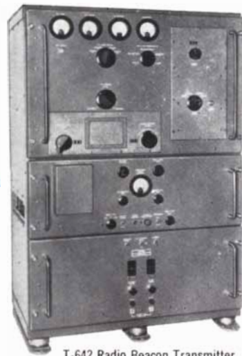
T-642 Radio Beacon Transmitter
