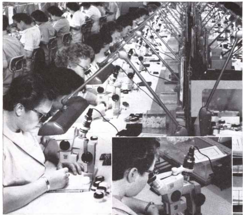
One of many assembly lines of skilled operators employing AO CYCLOPTIC Stereoscopic Microscopes to assemble advanced germanium computer transistors at Texas Instruments vast Semiconductor Components division in Dallas, Texas.
