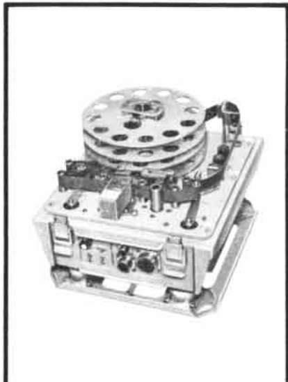
Need for greater accuracy in flight test analyses lead to development of this Honeywell airborne digital data recorder. Fast start-stop. 12 tracks on 3/4" tape. Coaxial reels hold 4 hours of recorded data.
