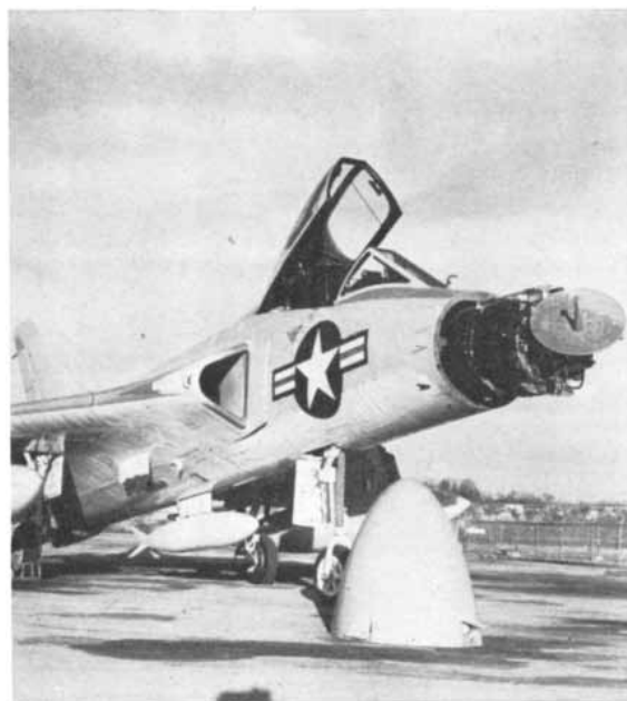
AIRBORNE ELECTRONIC SYSTEMS for weapons control, terrain avoidance, bombing and navigation, antisubmarine warfare, missile guidance, bomber defense and other applications are designed and manufactured by Westinghouse. Aero 13 Armament Control System, shown above, for the Navy's F4D Douglas Skyray fleet interceptor, is a recent example. Air Arm Division
