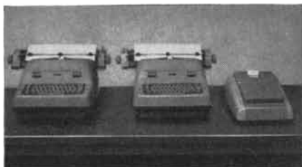
TWO TYPEWRITERS permit a single line log allowing columnar comparisons. Separate alarm printer records all off-normal variables.
