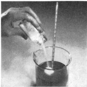
1. Into a liquid triglyceride such as cottonseed oil put a small percentage of monoglyceride made from any saturated fat.
