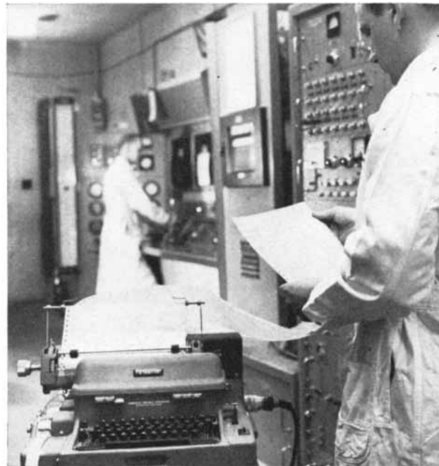
AUTOMATIC PRODUCTION TESTING, developed by Westinghouse, improves and speeds final pre-shipment testing. Test cell controls put engine through required tests automatically and record test results on the form prescribed for the engine log book.
