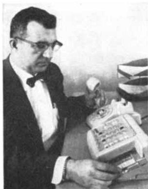
Original hand-made model of new data input device. Engineering now in progress at Western Electric will reduce the size of the unit to about that of a breast-pocket wallet.
