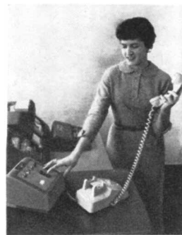
At the receiving end, operator can feed incoming data directly to the computer or into a standard card-punching machine simply by throwing a key.
