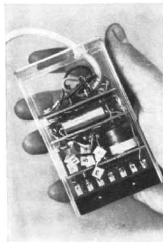
Western Electric engineers are miniaturizing this multi-frequency oscillator, the transistorized electronic heart of the new remote data input system. It makes use of low voltages normally used in telephone lines and requires no outside power supply.
