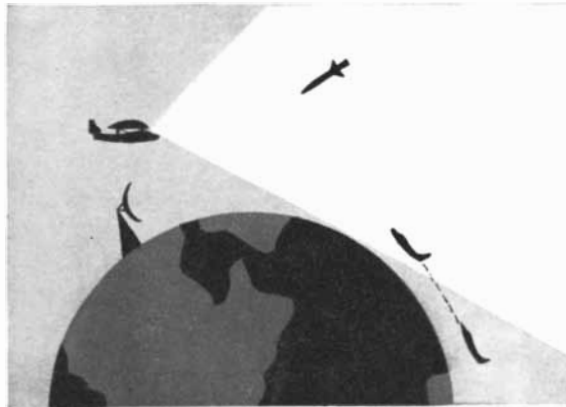
Detection range is increased appreciably when the radar detection equipment is airborne directly over the ground installation.
