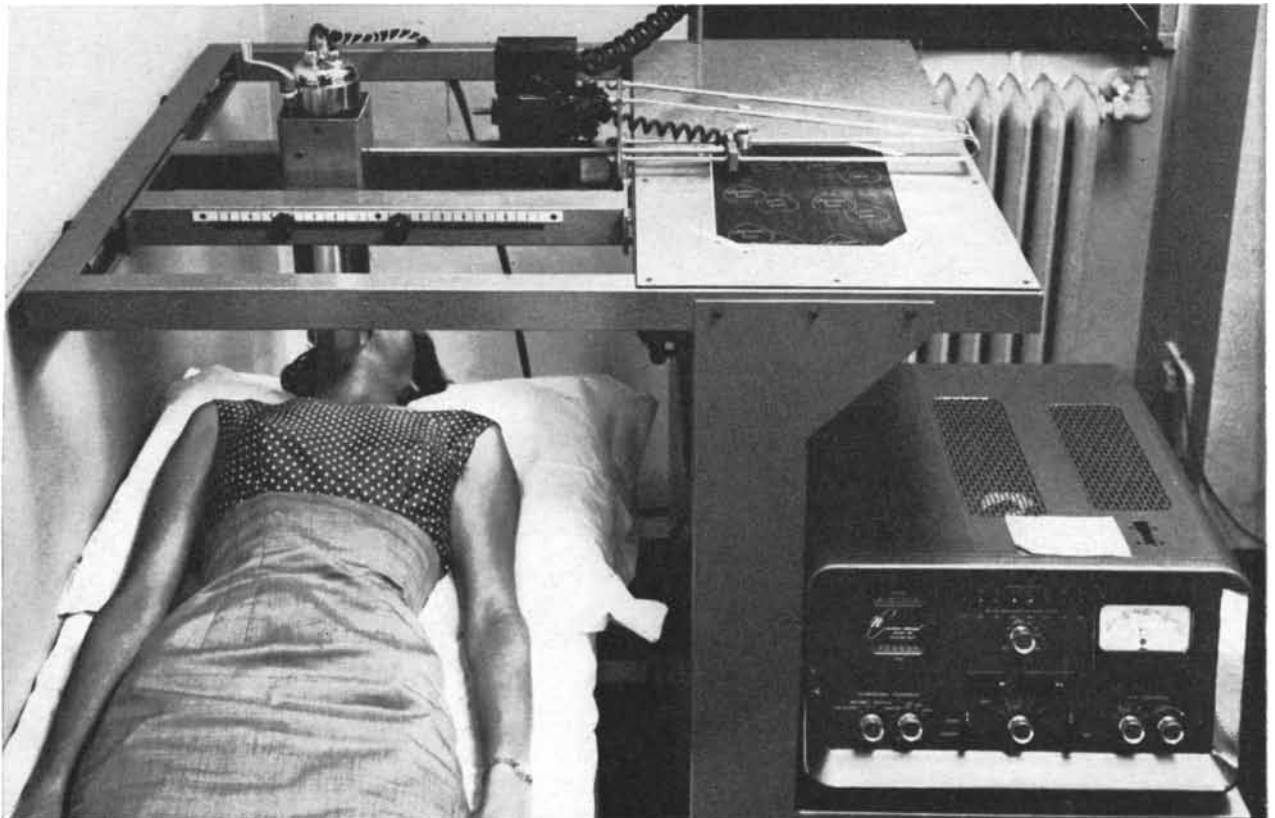
SCINTILLATION COUNTER DRAWS "MAP" of thyroid gland after patient has taken diagnostic dose of radioactive iodine solu-
