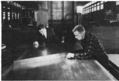
TOOLING PLATE, extra flat, is annealed to eliminate residual stresses.
