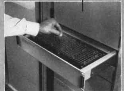
PINBOARD PROGRAMMING adds flexibility. You can change the logging or scanning sequence at will . . . substitute one type of input for another. Range, span, and zero adjustment are set by inserting pins in their proper places. No calculations are required. The pinboards are pinned in familiar units of measurements.
