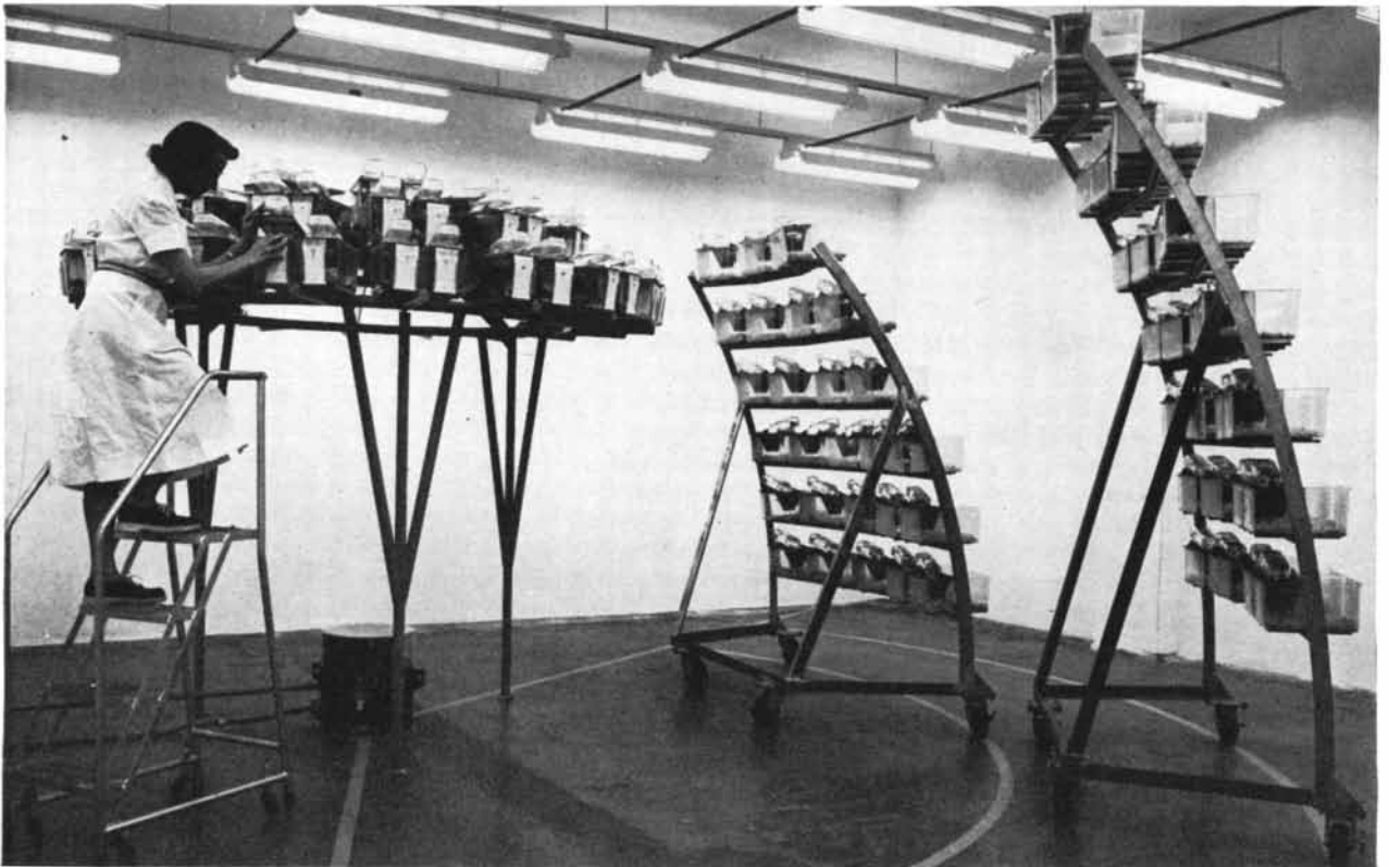
WHOLE-BODY IRRADIATION OF MICE is carried out at the Oak Ridge National Laboratory in this room. The cylindrical shielding-can on the floor contains a cobalt-60 source. The animals are placed in their cages on racks above and around the source.
