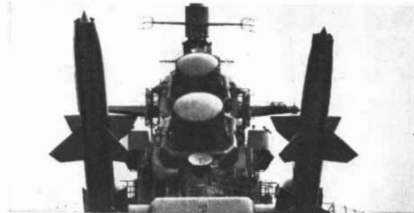
RESEMBLING SEARCHLIGHTS —radars aboard cruiser USS Galveston depend on power from Sperry microwave tubes to launch and guide Navy's Talos missiles on precise course at supersonic speeds.
