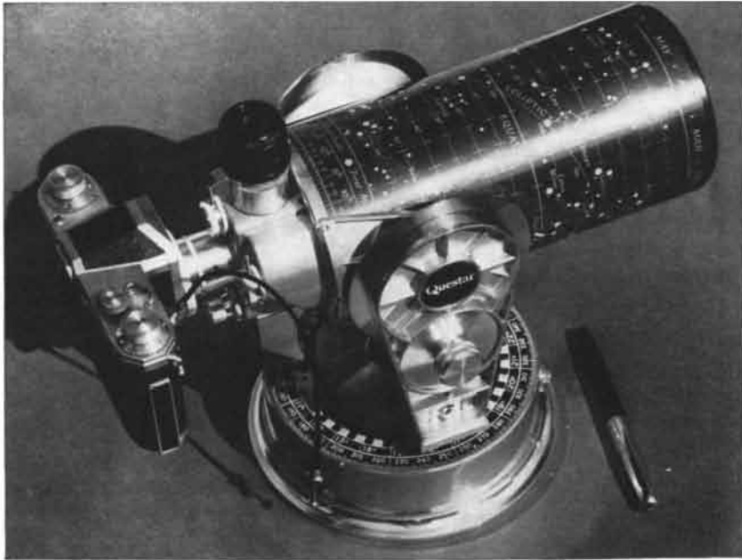
This is Questar with one of several suitable 35 mm. cameras attached. The telescope's 89 mm. aperture is always used wide open, since stopping down would only decrease the sharpness of this optical system.
