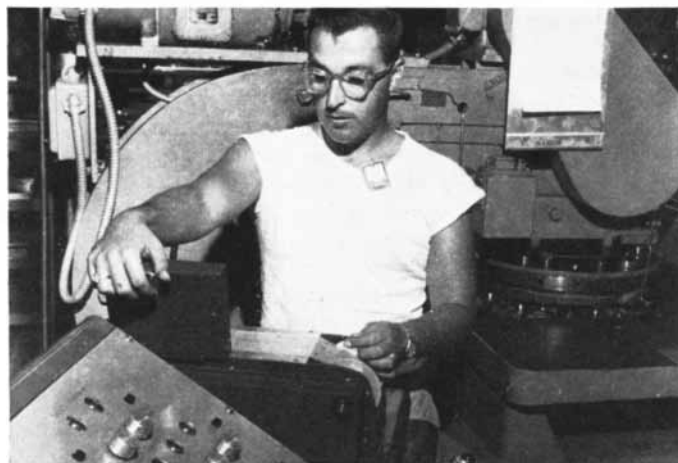
ADVANCED TECHNIQUES reduce costs and manufacturing time while maintaining high quality standards. Above, a Westinghouse-modified punch press at the Air Arm Division operates automatically by tape or dial control. It reduces lead time, cuts costs 60 to 70 percent over use of templates.
