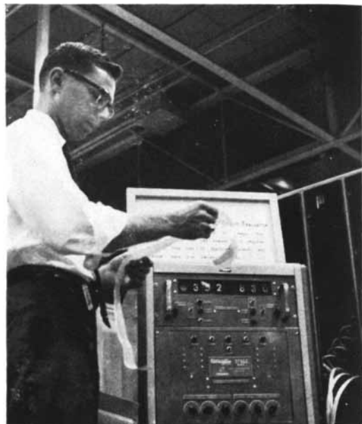
AUTOMATIC TESTING: Tape-controlled automatic equipment lowers test and inspection costs at Westinghouse defense plants. These controls are used in production as well as in environmental testing. Above, the Westinghouse-developed Self Programming Automatic Circuit Evaluator (SPACE) at the Electronics Division performs circuit tests 70 times faster than can be done manually.
