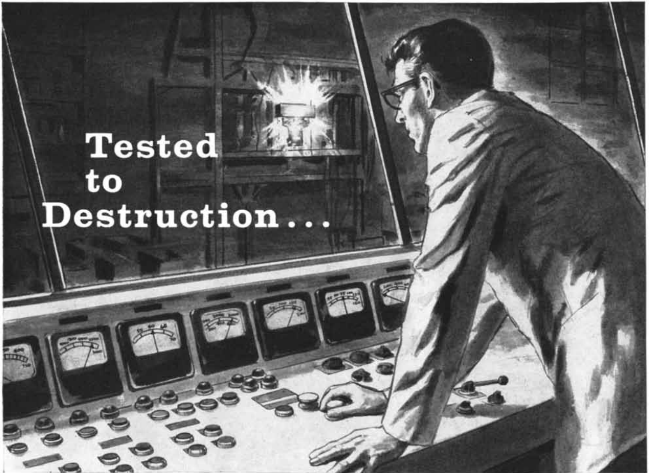
You're watching a motor starter "blow up" in the Allen-Bradley high current laboratory.
