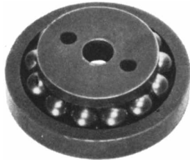
Unretouched photo of ball thrust bearing (shown actual size) after 250-hour test run without lubrication at 1000° F. Rings are M-2 tool steel; balls are tungsten carbide.
