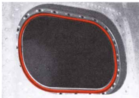
A similar application for Silastic, this time on the Army-developed Jupiter IRBM, another Chrysler-produced missile, is the seal on the angle-of-attack transducer compartment. Silastic was specified because it resists high temperatures encountered in re-entry.
