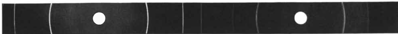
DIAMOND diffraction pattern indicates a cubic crystal. X-ray beam passed through holes in strip of film which surrounded the
