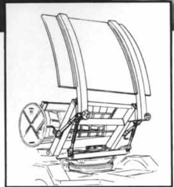
U.S. Army Signal Corps ground portable radar unit operated with two AiResearch electromechanical actuation systems.
