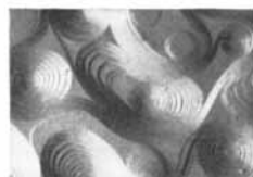
Reduction of Oxide Products (2500 x)
