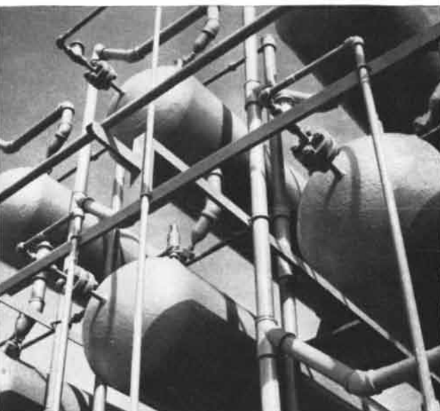
These pressure vessels for the U. S. Air Force Bomarc A system are seamless steel cylinders about 20 inches in diameter and 26½ feet long. The cylinder walls are slightly more than an inch-and-a-half thick and will contain gas at pressure up to 4500 psi.
