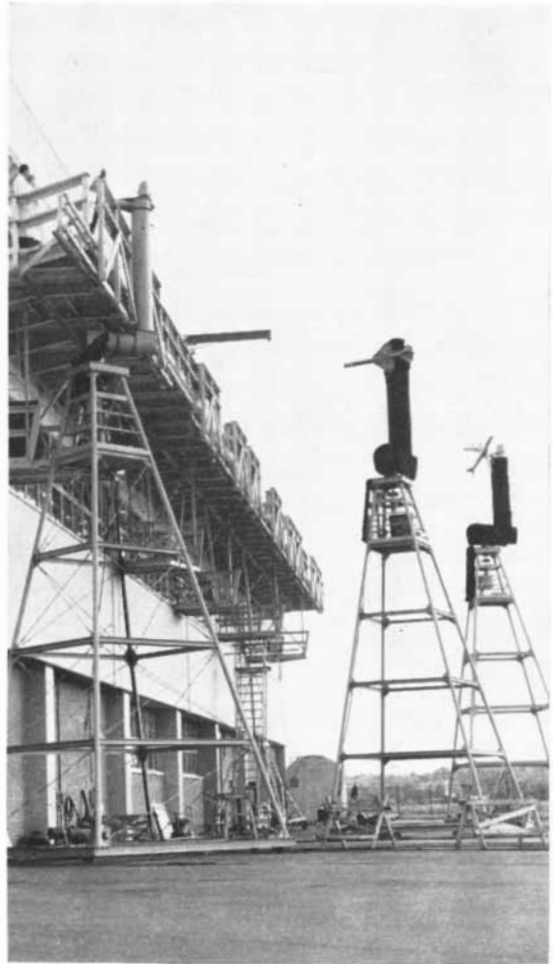
ANTENNA PATTERN RANGE, with movable towers capable of handling models up to 1000 pounds. Boeing has openings in ECM antenna development, and in gas, solid and liquid dielectric research, as well as large-aperture antennas for ASMs, orbital vehicles and airborne warning systems. Other openings are available in instrumentation, missile guidance and control.
