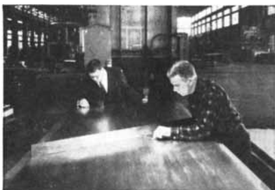
TOOLING PLATE , extra flat, is annealed to eliminate residual stresses.
