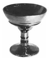
Silicon crystal chalice, produced by combining growing and casting techniques, illustrates capabilities of TI giant crystal puller that grows 10-in. silicon crystals and casts  $\frac{1}{2}$ -in. plates to 12-in. diameters.
