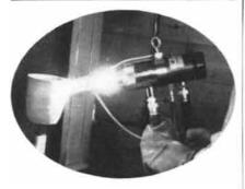
Apply coatings of high melting point materials such as tungsten, tungsten carbide, molybdenum, chromium carbide, titanium oxide, rare earth oxides. Operates at 10,000°-15,000° F.
