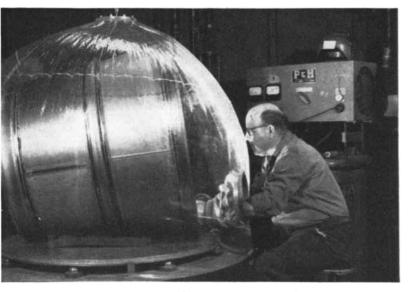
Welding of titanium at P&WA is based on the company's experience in production of more than 5800 jet engines containing titanium parts. Weld strength of beta titanium alloy is considerably improved by cold working the weld.
