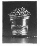
This thimble—actual size—greatly magnified on the left, contains 1,053 PSI Micro-Diodes. The standard subminiature diode is shown below. (Photos by Don Mannix.)
