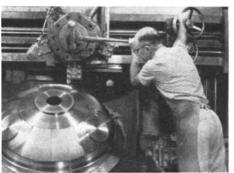
Flow-turning from roll-forged rings, makes feasible production of fullscale titanium rocket cases, since it yields integral cylinders, eliminates need for longitudinal welds, conserves input metal.
