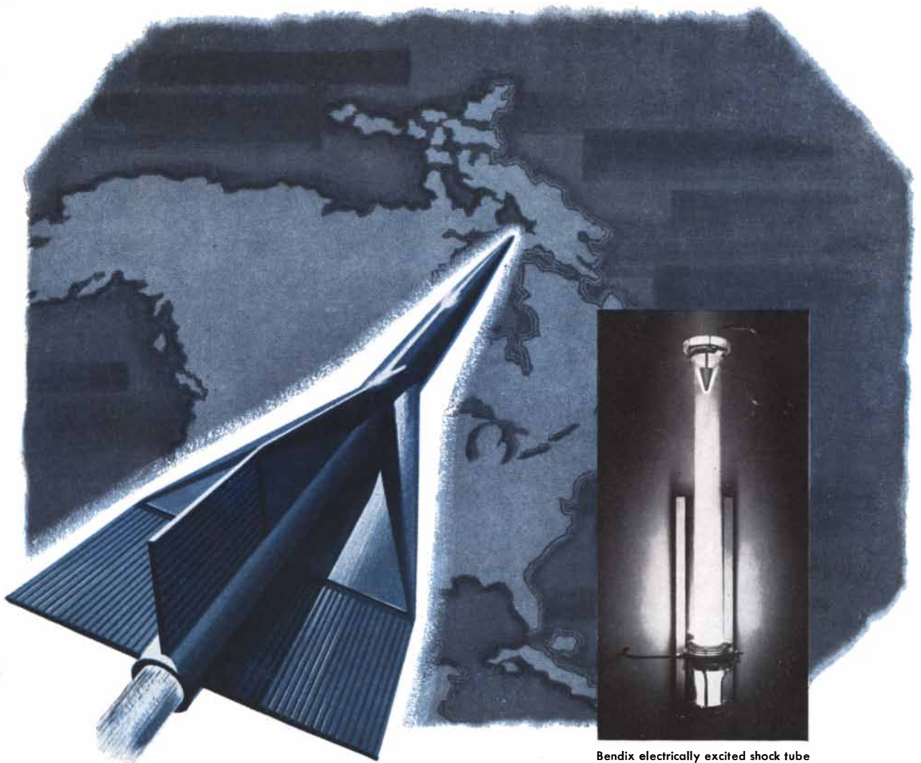
Bendix electrically excited shock tube can be photographed by illumination from hot gases.
