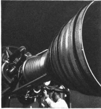
Thin-wall nickel tubing, used in the fabrication of thrust chambers for the Atlas, Thor and Jupiter missiles, meets exacting design requirements and survives extremely severe fabrication, test and operational conditions
