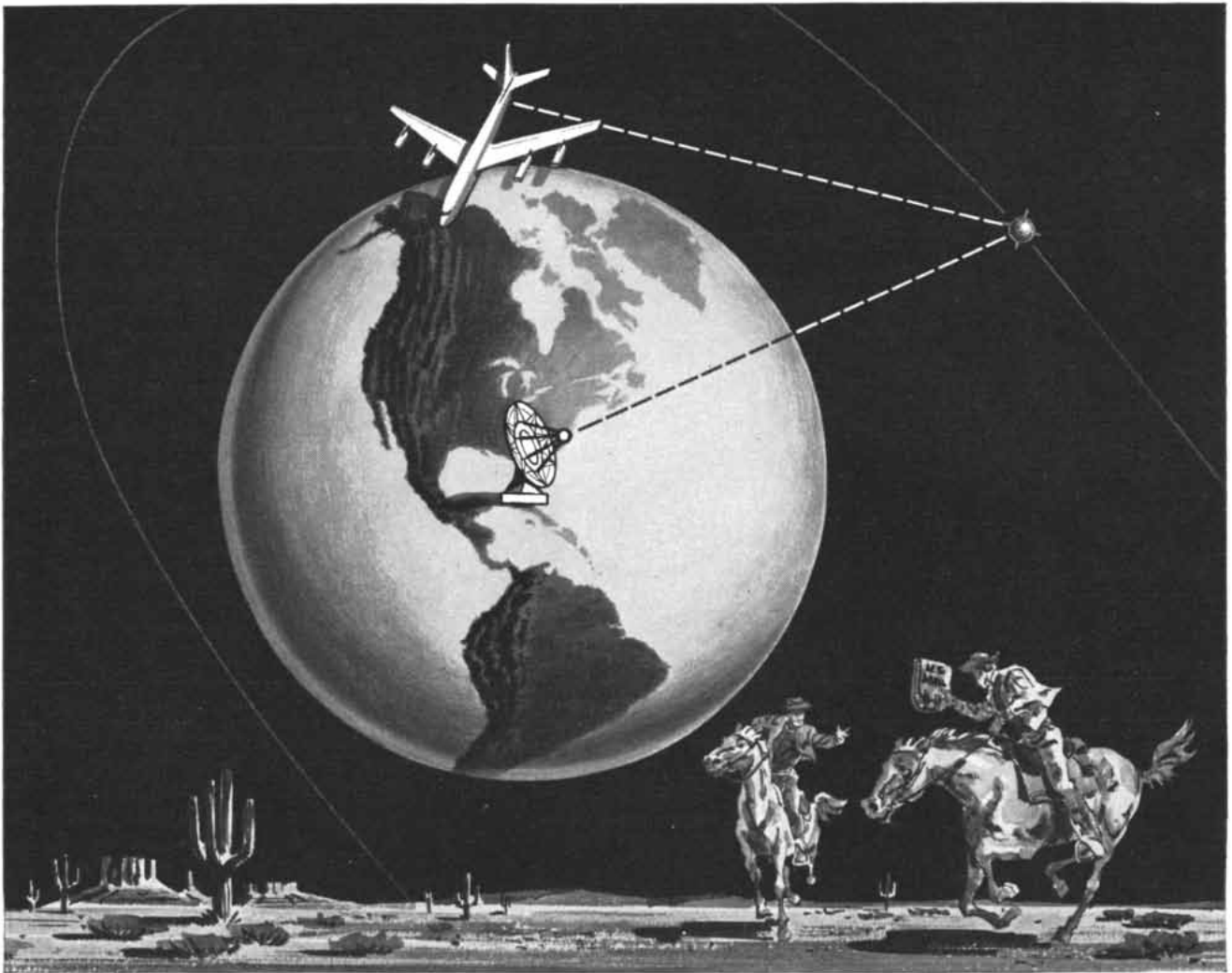
Illustration shows how satellite is used as relay station for two-way radio messages between Air Force station on earth and bomber in flight.
