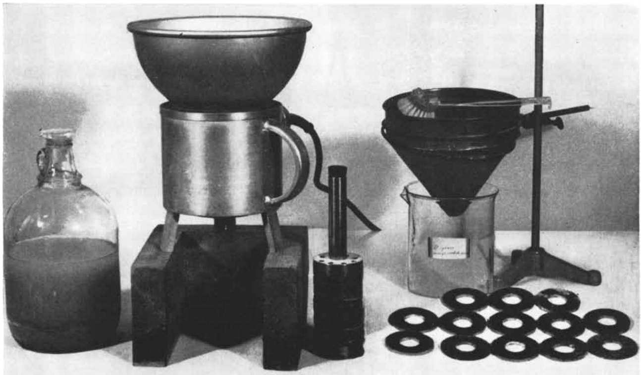
ELECTROMAGNETIC APPARATUS is used by author to collect cosmic spherules. At left is suspension of sediment, which is poured into apparatus next to it. In use the apparatus contains the electro-
