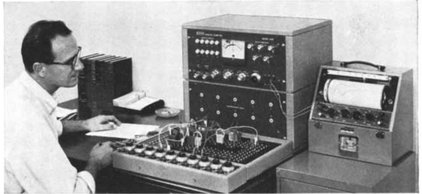
The Donner 3400 Desk-top Computer functions as a compact, versatile electrical model of a dynamic system.
