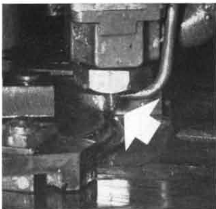
Machines equipped with the new Kennametal hard carbide nozzles spray sealing material on can lids—at a 90% saving in nozzle cost.
