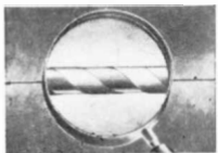
Hair-Like Twistor Wire, magnified 33 times, forms heart of new electronic computer memory device.
