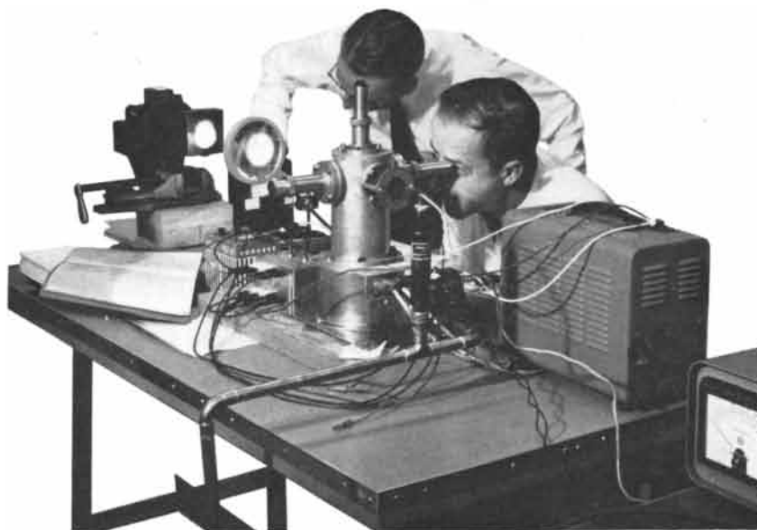
An electron device permits scientists to study the behavior of charged dust particles held in suspension.
