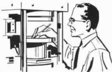
Battelle modified Bridgman anvil for combined high-temperature, high-pressure studies. This configuration has been used for material studies to greater than 3,000,000 psi.
