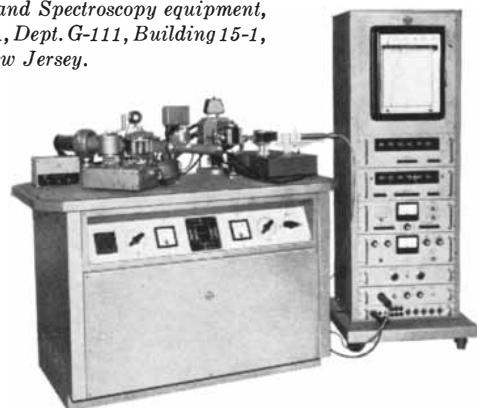
Vacuum Spectrometer and a Diffractometer mounted on Crystalloflex IV and connected to Electronic Circuit Panel
