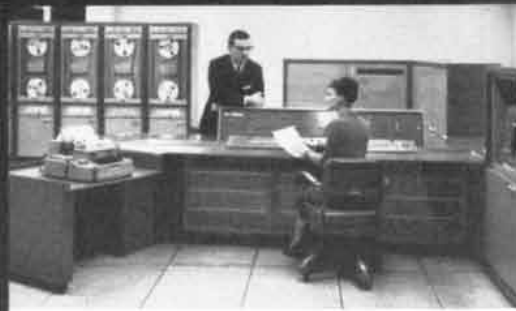
PHILCO 2000 DATA PROCESSING SYSTEM. World's First in All-transistor Logic and Circuitry.
