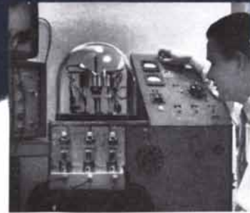
Bearingless support using electric fields
