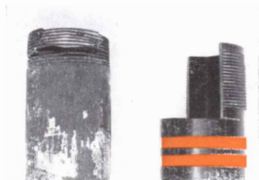
Fibercast Tubing (right) used to suspend a 1,200 lb. pump for 3 years in a salt water supply well. There was no loss in strength. The damaged plastic-coated steel nipple (left) was used in the same installation, failed after 3 months' service.
