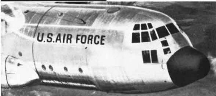
Cored deicing radome, built by GAC for C-130
