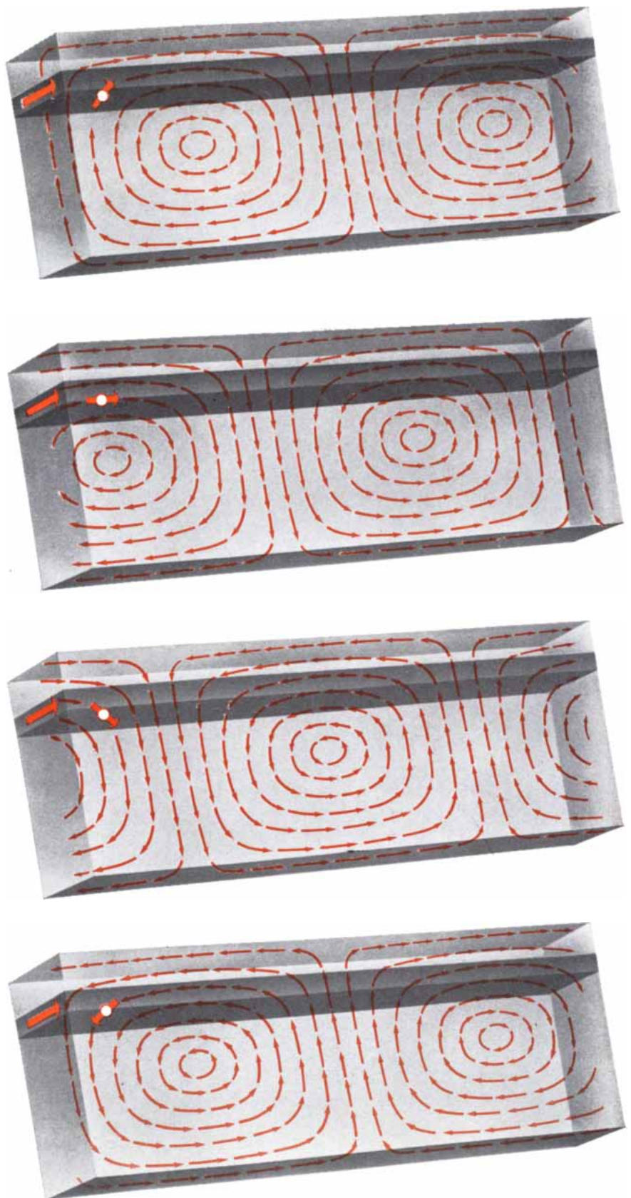
ISOLATOR is made of a section of rectangular wave guide containing a piece of ferrite (dark gray object near top of wave guide). Successive drawings show advance from right to left of a magnetic field pattern (broken colored arrows) through wave guide. Colored arrow through white dot at top left in wave guide shows direction of field at that point. Colored arrow at left edge represents "biasing" field from external coil (not shown).
