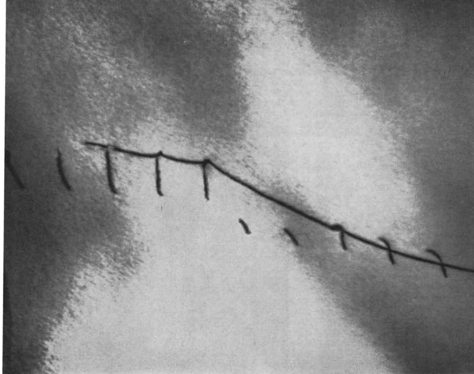
Structural imperfections, represented by this dislocation network in thin tantalum foil, determine the properties of a superconductor (electron transmission; 64,000x).
