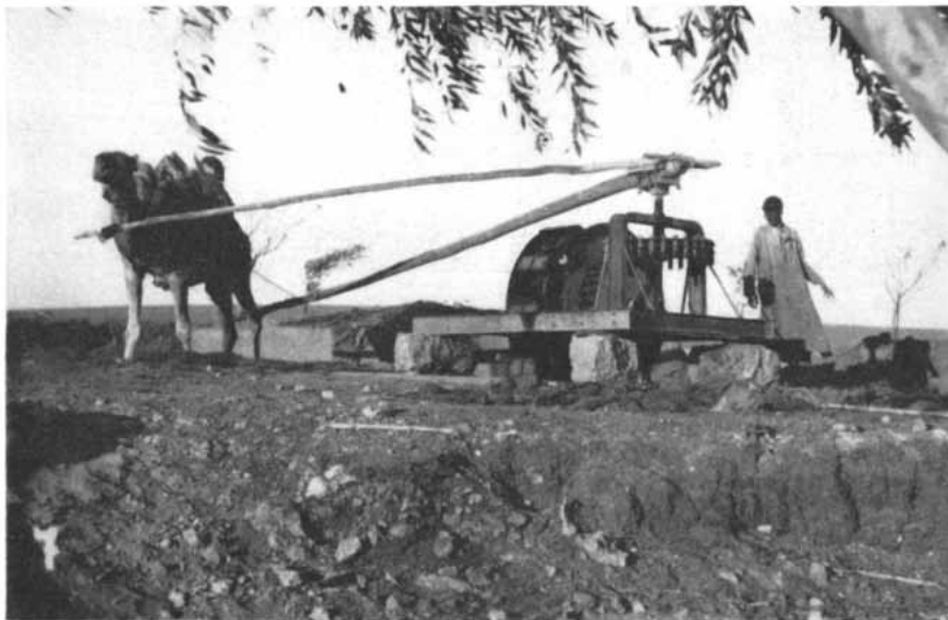
WOODEN WATER-WHEEL , powered by camel, lifts water from main irrigation ditch into feeder ditches to bring water to fields in valley of the Euphrates in northern Syria.
