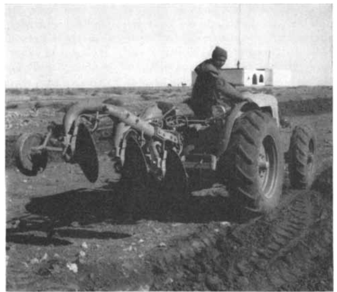
STEEL DISK-PLOW , drawn by tractor, has not succeeded everywhere in Mediterranean, whose soils must be handled with care.
