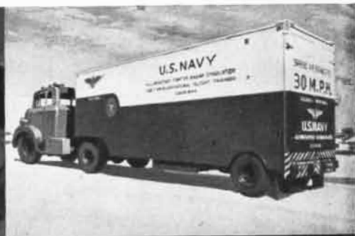
Mobile flight simulator — built by GAC for Navy.
