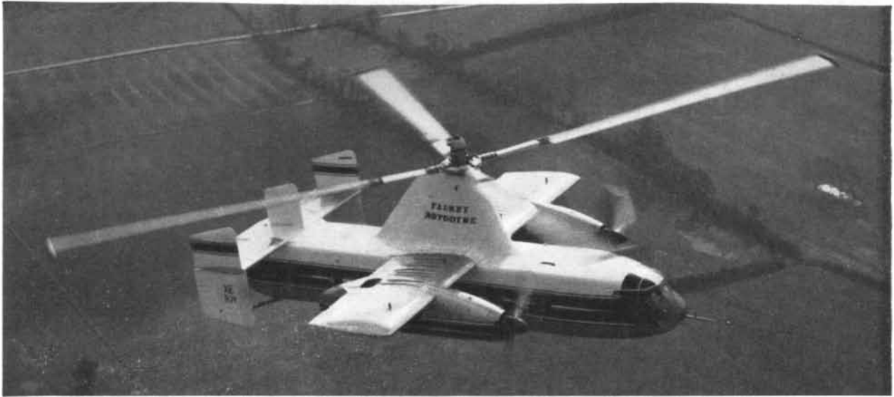
FAIREY ROTODYNE is a dual-propulsion VTOL airplane. The rotor above the fuselage provides thrust for vertical flight; the
