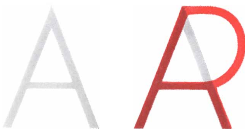
TEMPLATE MATCHING cannot succeed when the unknown letter ( color ) has the wrong size, orientation or position. The program must begin by adjusting sample to standard form.
