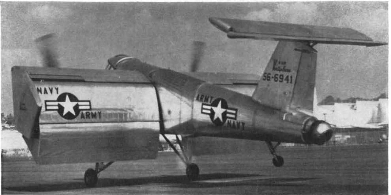
THRUST-DEFLECTION AIRPLANE was built by the Ryan Aeronautical Co. The large flaps, when turned downward, bend the
