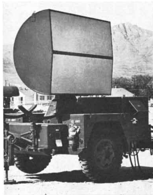
This continuous wave acquisition radar picks up targets down to tree-top levels.
