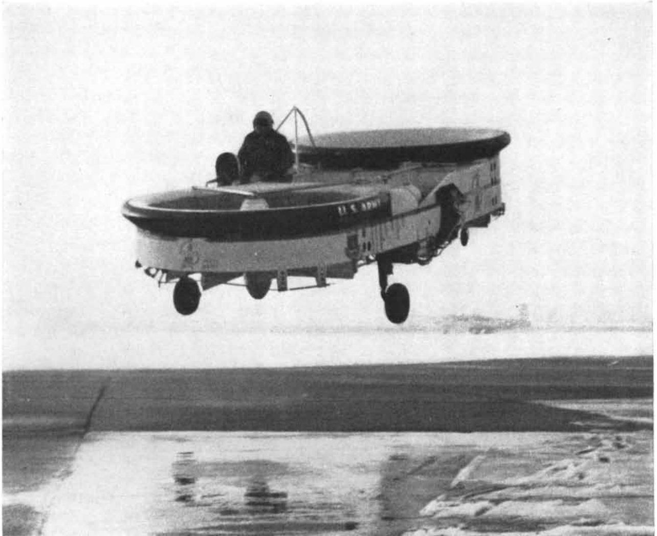
PIASECKI "AERIAL JEEP" derives thrust from ducted fans mounted rigidly to the air frame. To fly horizontally the entire
