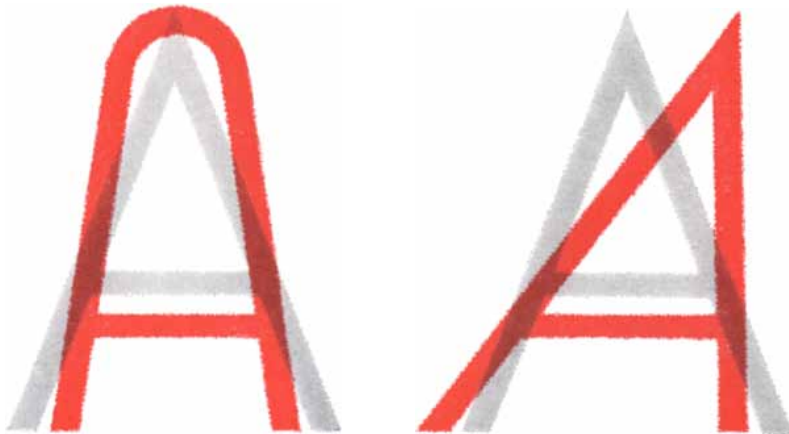
INCORRECT MATCH may result even when sample ( color ) has been converted to standard form. Here R matches A template more closely than do samples of the correct letter.
