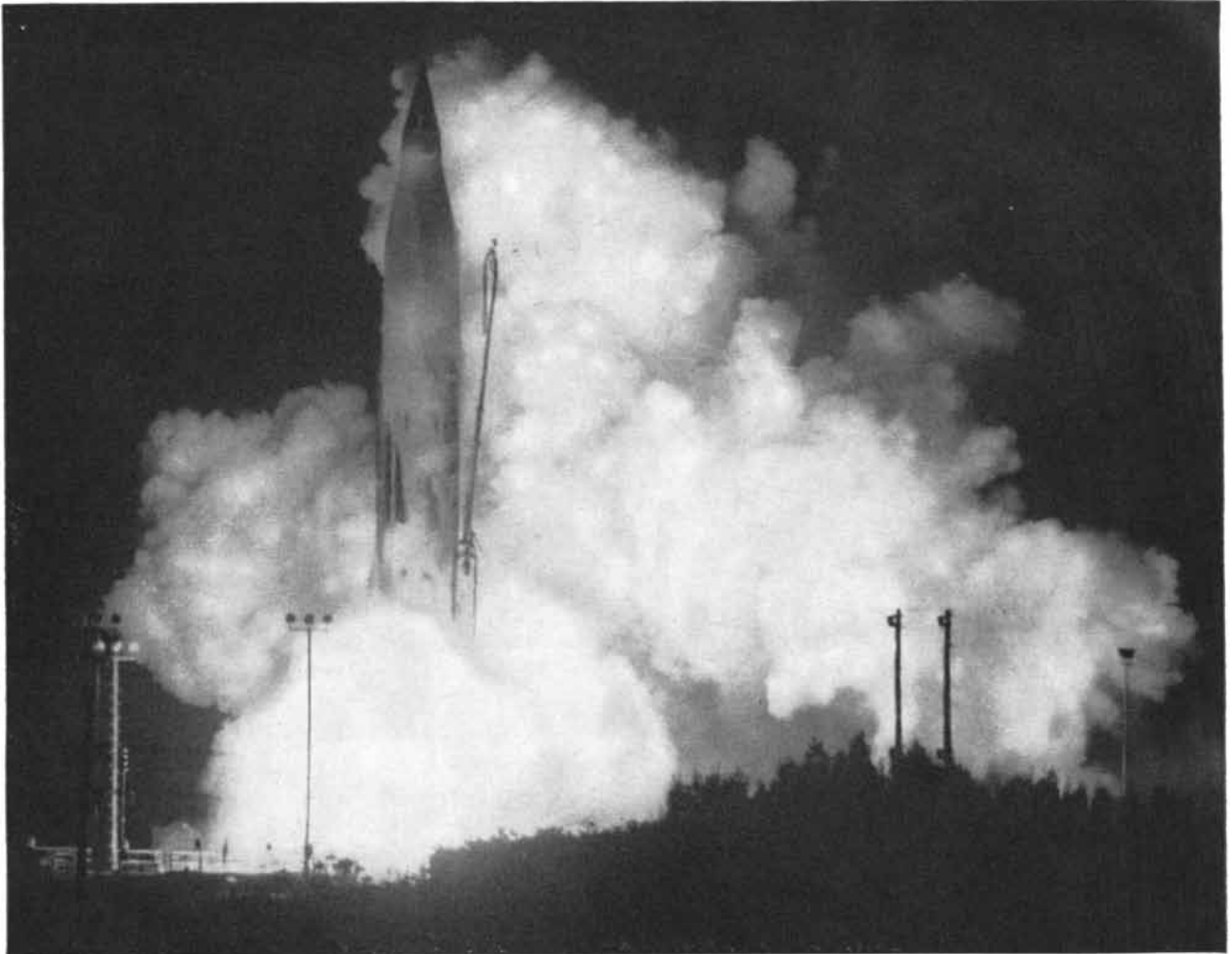
Record breaking Atlas missile billows flame and vapor as she launches 4¼-ton satellite into orbit. Constructed of Type 301 Nickel Stainless Steel, Atlas is built by Convair (Astronautics) Division of General Dynamics Corporation. U.S. Air Force photo
