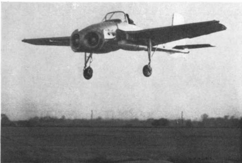
BELL X-14 is a turbojet design using thrust deflection to provide lifting force for takeoff and landing. The tail pipes beneath the wing can be directed horizontally or vertically.
