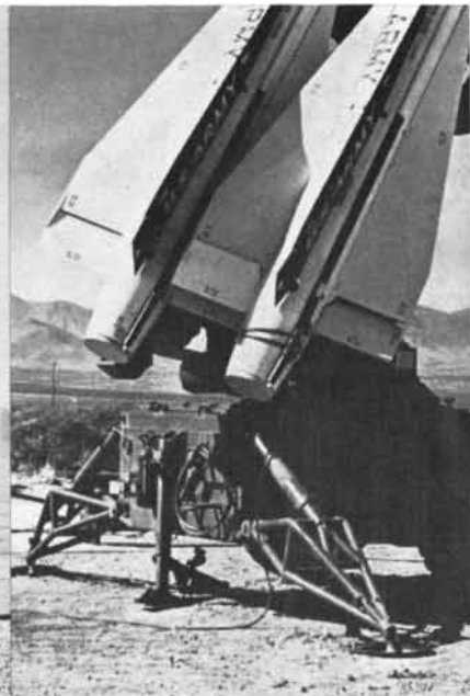
Tubular outriggers give the launcher good stability with maximum weight conservation.
