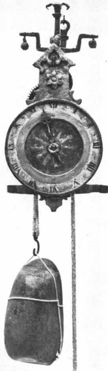
GOTHIC CLOCK , dating from the early 16th century, was photographed at the Smithsonian Institution. Stone at bottom is the driving weight; arm at top is part of escapement. Clockworks were among earliest examples of well-ordered machines.
