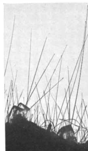
In the above electron micrograph, oxide "whiskers" are seen to erupt from stainless steel after reaction with oxygen. By pre-stressing the steel and adding a trace of chloride ion in water vapor, the crystal habit changes and upright parallel plate crystals appear.
