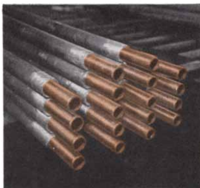
Lead surfacing removed from ends of Cupralum tubes preparatory to insertion in lead-clad steel tube sheet. Tube ends are usually rolled, but for severe thermal cycling service, may be brazed to outer steel face of tube sheet.
