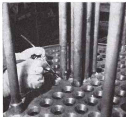
Lead surfaces of Cupralum tubes and of tube sheet are fused by lead-to-lead welding. Then an extra thickness of lead is applied at the joint for extra protection.
