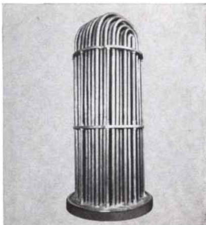
Two U-bend Cupralum tube bundles like this are used in a Ferrolum (lead-surfaced steel) separator tower to boil off ammonia from a urea carbonate ammonia solution—in the production of urea fertilizer. Anaconda copper tube core 1" O.D., 12 gauge, handles 150-lb. steam. Lead surface is \frac{3}{16} " inch thick. Separator tower operates at 145 C (293 F) and 240 psi.
