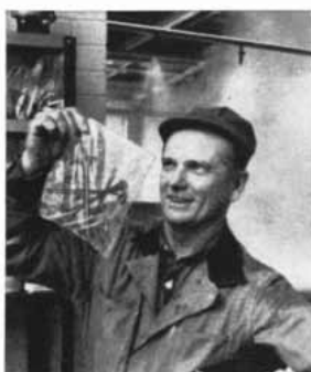
3. Volatile corrosion-inhibitor packages of "Mylar" fight rust, offer easy identification of parts.
