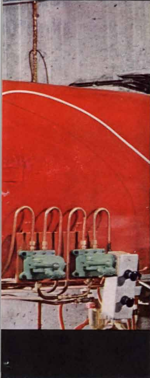
The Supply Lines: 230 spaghetti-like cables converge in rear of cannon to deliver peak currents to 4,000,000 amps.
