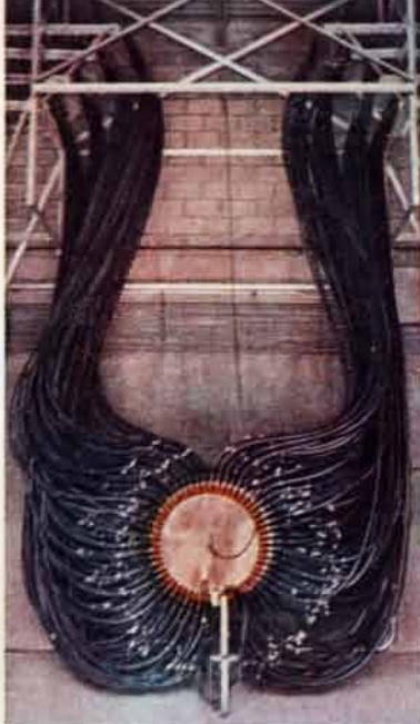
The Supply Lines: 230 spaghetti-like cables converge in rear of cannon to deliver peak currents to 4,000,000 amps.
