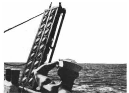
About to be submerged, this Bendix-developed "underwater sound source" transmits sound waves beneath the sea. It is designed to increase sonar capabilities.
