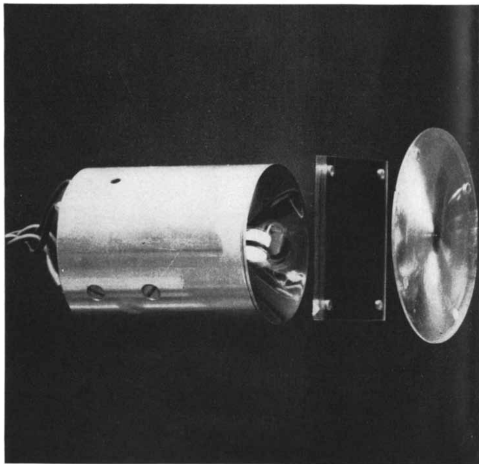
RUBIDIUM IS PUMPED by beaming light from a rubidium-vapor lamp ( far left ) through a circular polarizer ( square at left center ) and a plastic condensing lens into an
