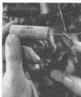
3. Capacitors with insulation of "Mylar" give long-lasting reliability . . . need for costly encapsulation is eliminated.
