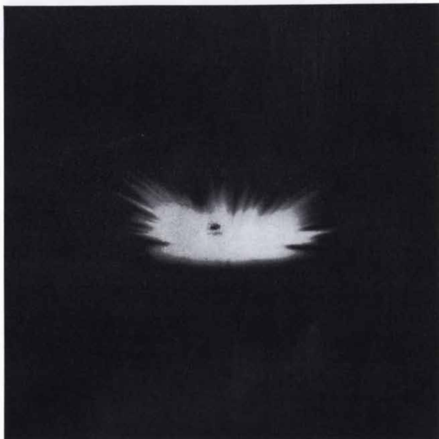
FLASH OF LIGHT accompanies impact at high speed in a helium atmosphere. Target is seen almost head-on ( top ) and from side ( bottom ). Dark spot in top photograph is impact crater. Photographs show a steel sphere striking a copper target at 10,000 feet per second.
