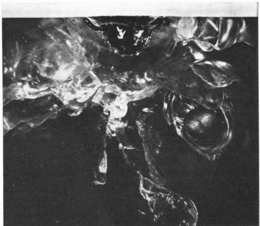
TRANSPARENT TARGET of epoxy resin shows extensive region of fracturing after being struck by nylon sphere. The sphere was about 1/4 inch in diameter and was fired at a velocity of 21,000 feet per second. The crater shown in this profile view is about 2/5 inch deep.
