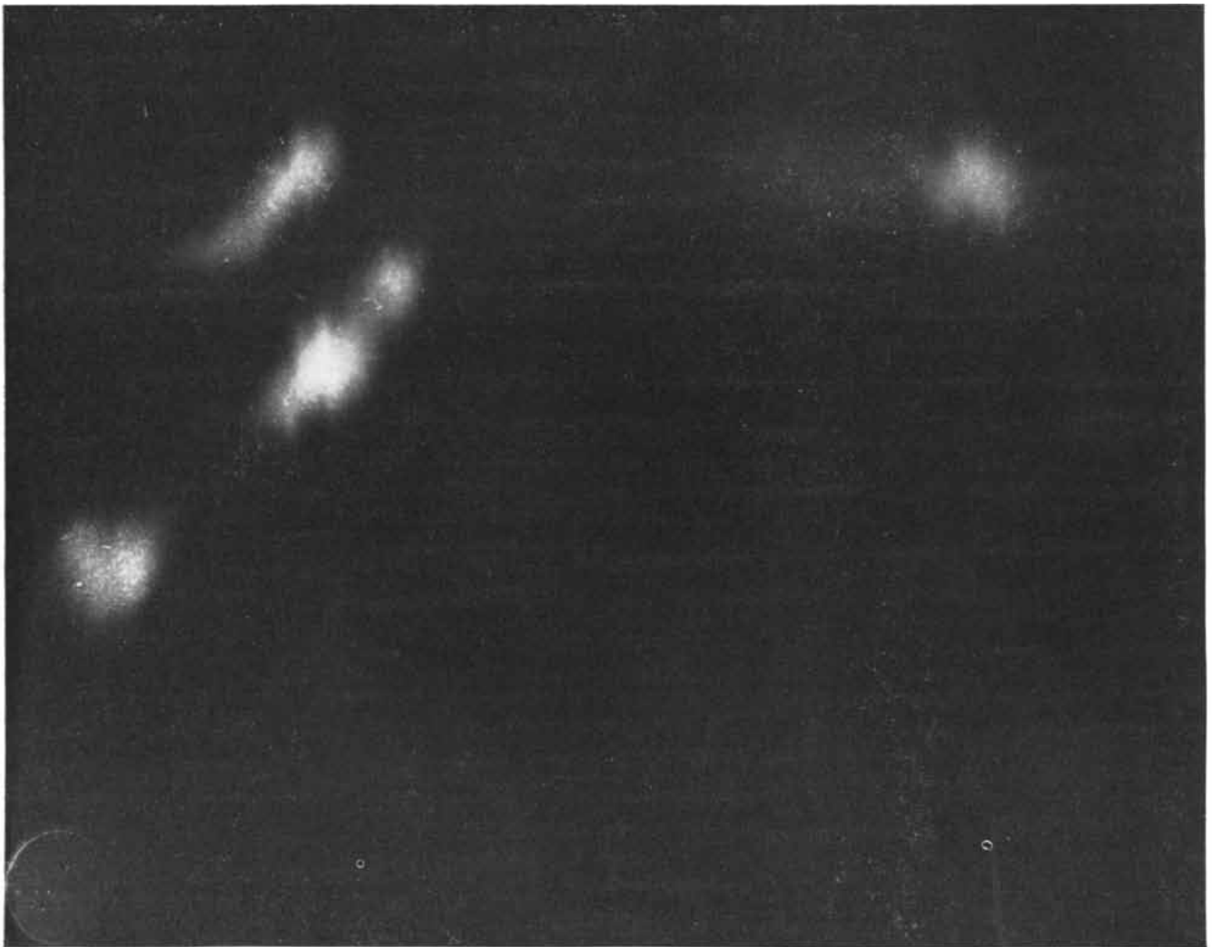
RADIOAUTOGRAPH OF A CHROMATOGRAM is used to analyze products of photosynthesis by isolated chloroplasts. A sample of the reacting mixture is placed on moist chromatogram paper at spot in lower left corner. The various compounds then
