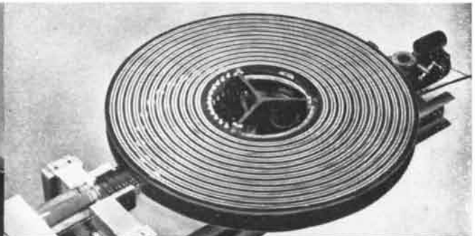
5. Large slip-ring assembly built by GAC.
