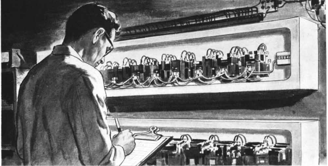
This engineer is "reading" the number of millions of trouble free operations on Allen-Bradley industrial relays on accelerated life tests.
