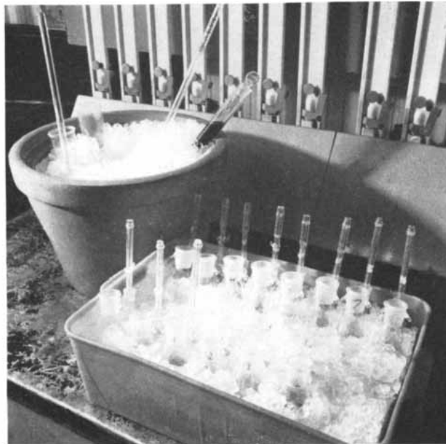
ISOLATED CHLOROPLASTS in stoppered cylinder in bowl at left are placed in vessels having long tubes (foreground) along with the reagents that contain radiocarbon or radiophosphorus.
