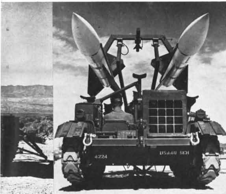
The Loader-transporter has an extremely low silhouette. It weighs only 5,250 pounds.
