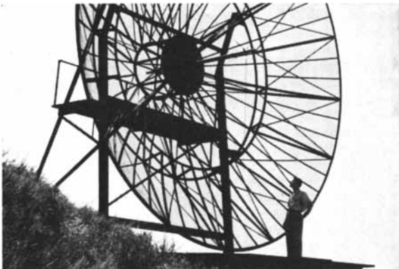
This giant transmitting antenna creates the beam for experimental antenna pattern measurements – part of the Hughes microwave research and development programs.
