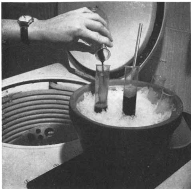
FILTRATE IS Poured INTO TEST TUBES which will be placed in a refrigerated centrifuge. Spinning the material at high speed separates the chloroplasts from the other portions of the cells.
