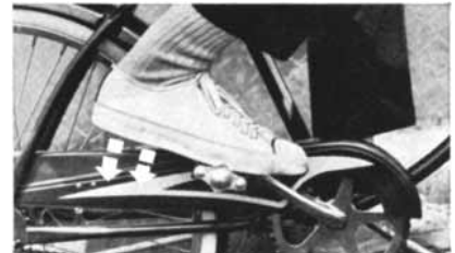
Changing gears is easy with the new Bendix automatic gearshift bicycle brake. The rider merely back-pedals a couple of inches, then pedals forward in the desired gear.
