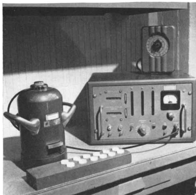
RADIOACTIVITY IS MEASURED by placing planchet in apparatus at left. Machine at right registers counts, showing the amount of radiocarbon or phosphorus absorbed in photosynthesis.
