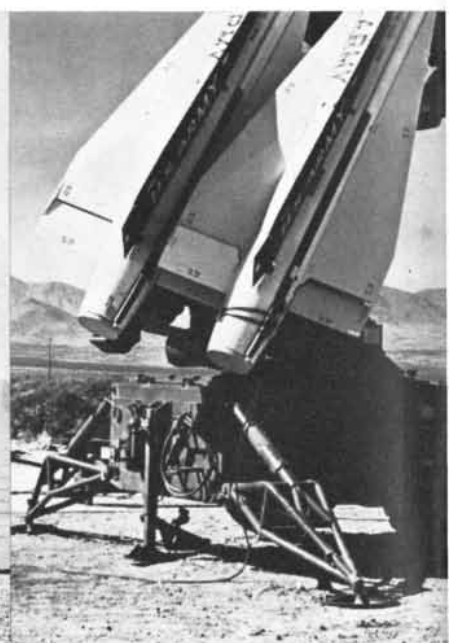
Tubular outriggers give the launcher good stability with maximum weight conservation.
