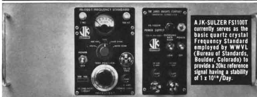
Total Dimensions, Standard and Power Supply: 7½" W x 6" H x 12½" D. Shown mounted in 7" x 19" rack panel.
