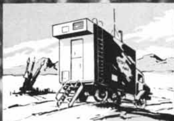
Trailer mounted refrigeration unit, 5 tons capacity
