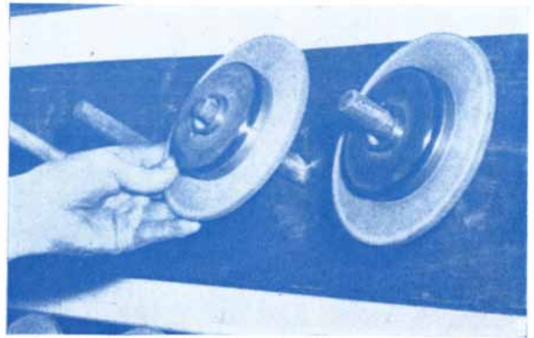
A specially developed type of grit enables resin-bond diamond wheels to grind rapidly and efficiently.
