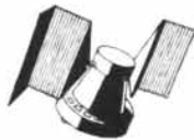
Project Aeres —24-hour stationary weather satellite. Launched in equatorial orbit. Three satellites could permit continuous observation of most of earth's surface.
