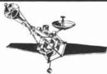
Project Mariner —600 to 1200 lbs. First U. S. Planetary missions to Venus and Mars. Modified craft for hard landings on moon.
