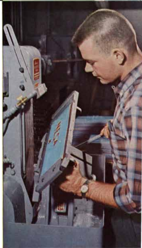
After forming, the thin layer of color is sanded away from certain raised areas to expose the second color underneath.
