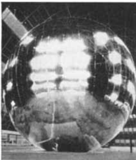
1. Huge (100 ft. diam.) inflatable satellite of metalized "Mylar" stays strong and flexible in sub-zero outer space.
