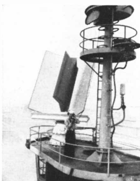
High over the deck of the missile cruiser USS Galveston, this new Hughes 3-D radar antenna simultaneously detects the range, bearing and altitude of a great number of targets. The sailor shows comparative size.
