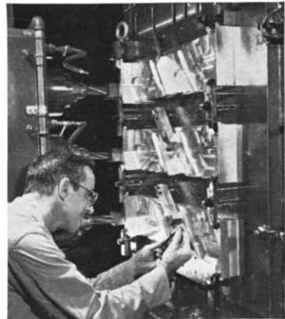
Three-spindle Keller mill simultaneously machines three B-52 wing structural members under direction of Bendix numerical control system. Saving in flow time: 4 weeks.
