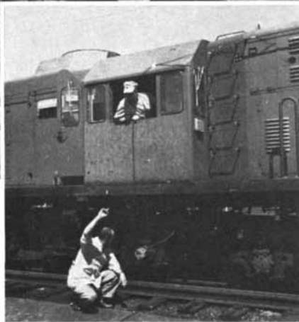
Measurements engineer with General Electric Locomotive and Car Equipment Department checks operation of PI recorder in locomotive cab.
