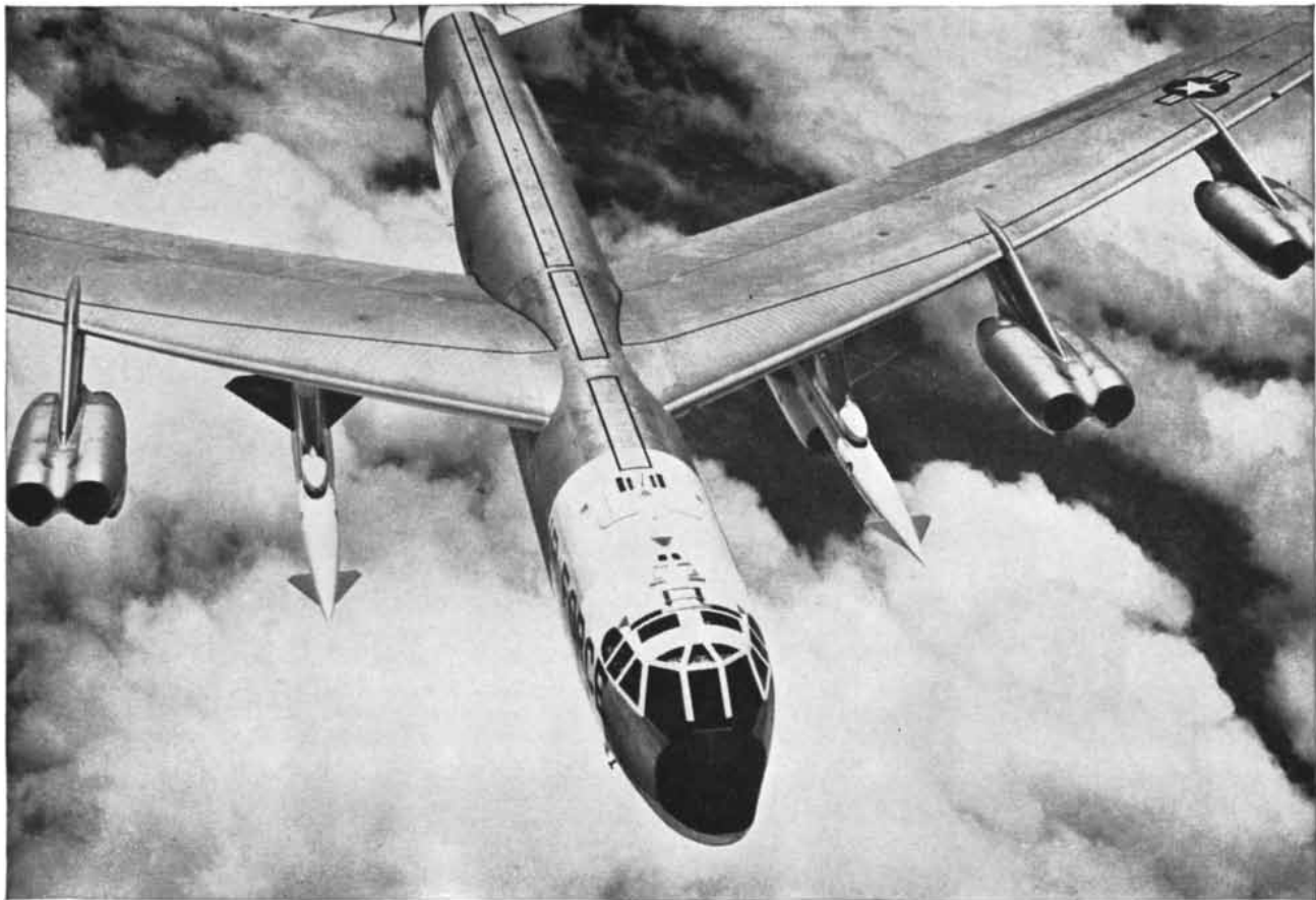
The Air Force's eight-jet Boeing B-52G Stratofortress has a non-refueling range of over 9,000 statute miles, enabling it to span oceans and still return to U.S. bases.
