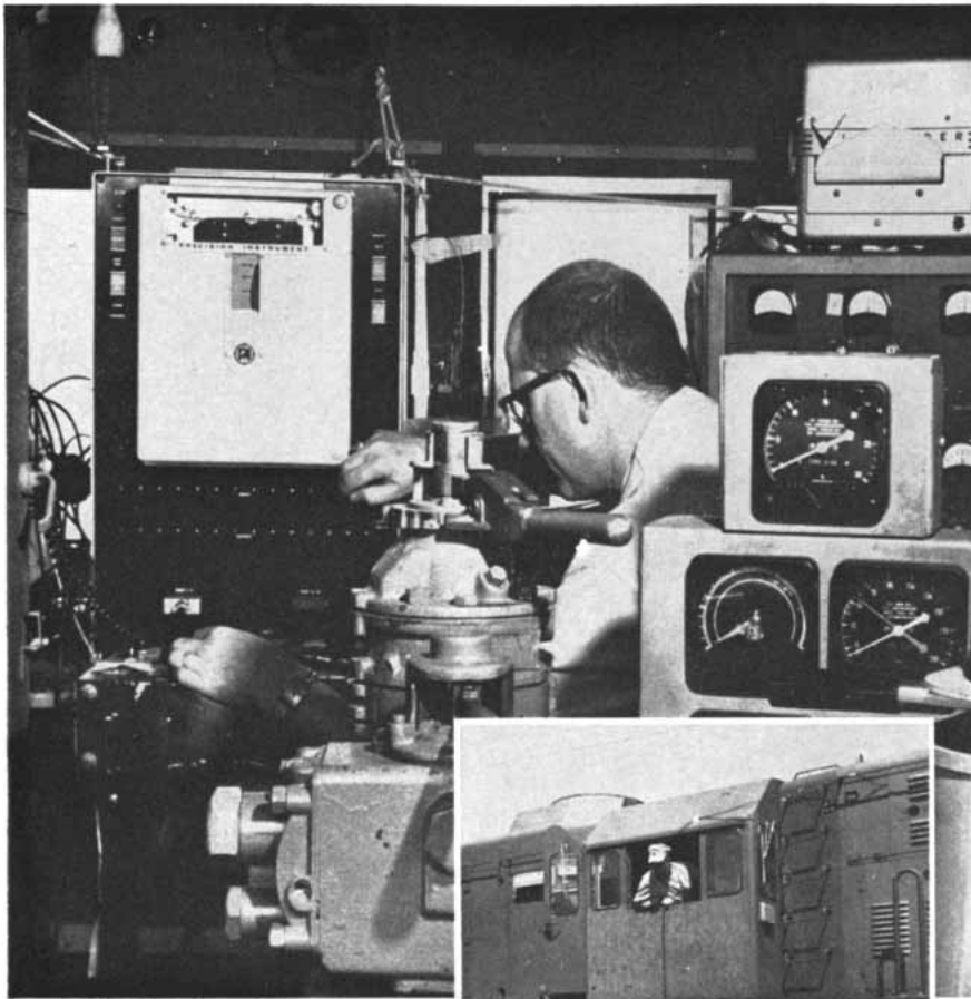
Measurements engineer with General Electric Locomotive and Car Equipment Department checks operation of PI recorder in locomotive cab.
