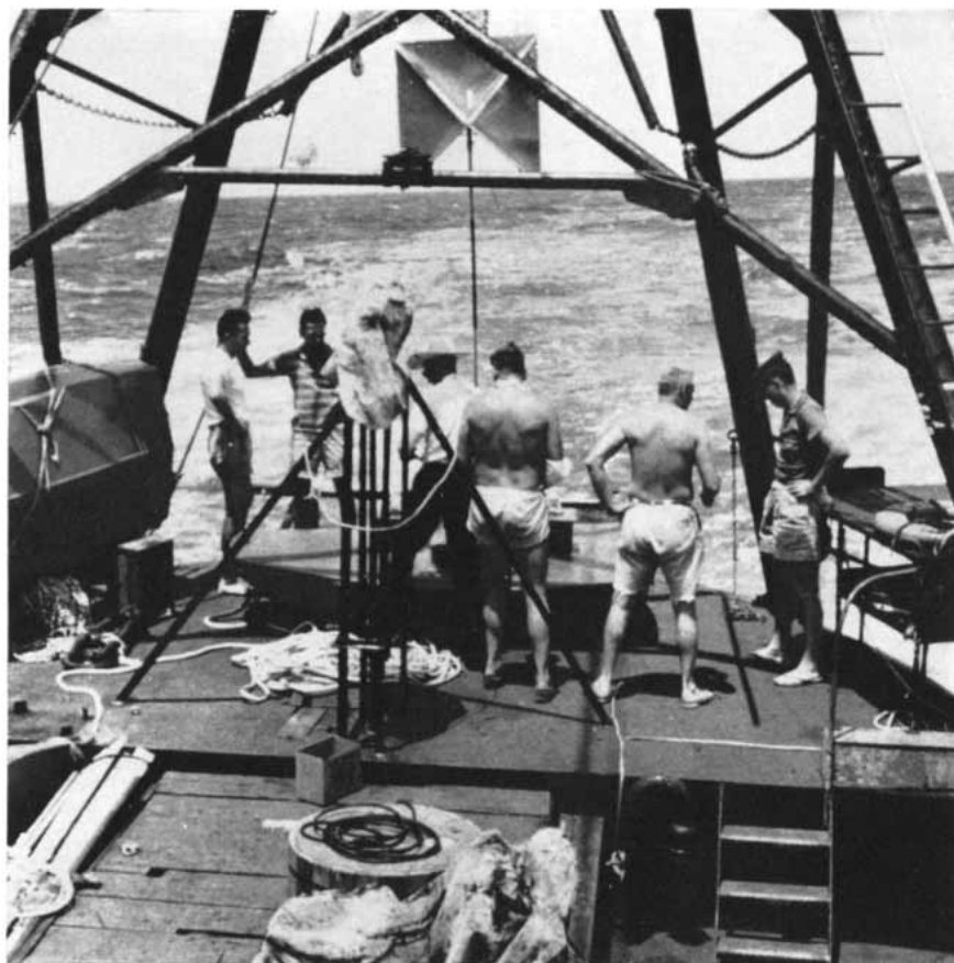
BUOY MARKER is launched over the stern of Horizon for the first time as the expedition begins its observations. The marker provided a reference point for measuring the drift.
