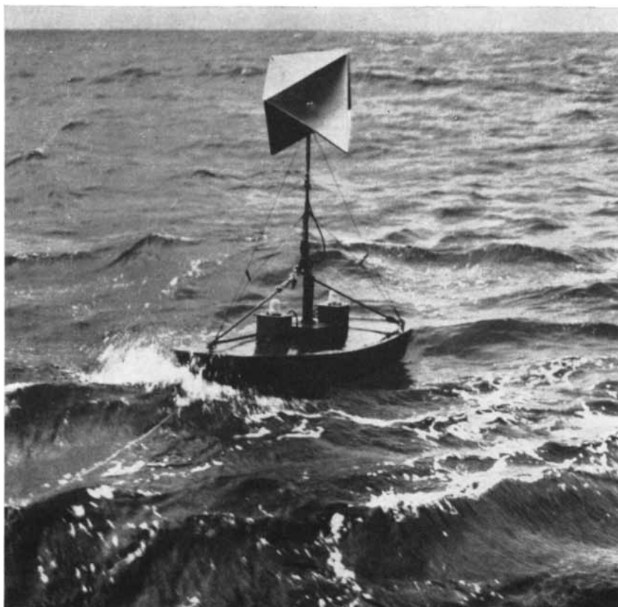
MARKER RIDES AT ANCHOR in mid-Pacific. The marker, an eight-foot pram, is moored by the line at left to the taut-wire buoy. The pram carries a metallic target for radar tracking.
