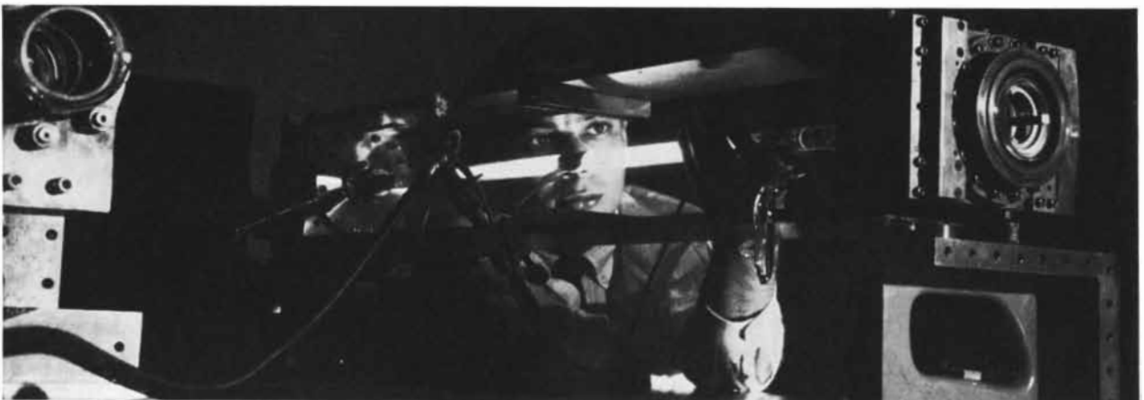
The Optical Gas Maser (above) was first demonstrated at Bell Telephone Laboratories. Heart of unit is a 40-inch tube containing helium and neon. Interaction between gas atoms produces a continuous, coherent beam of infrared light that may one day be used in communications.
