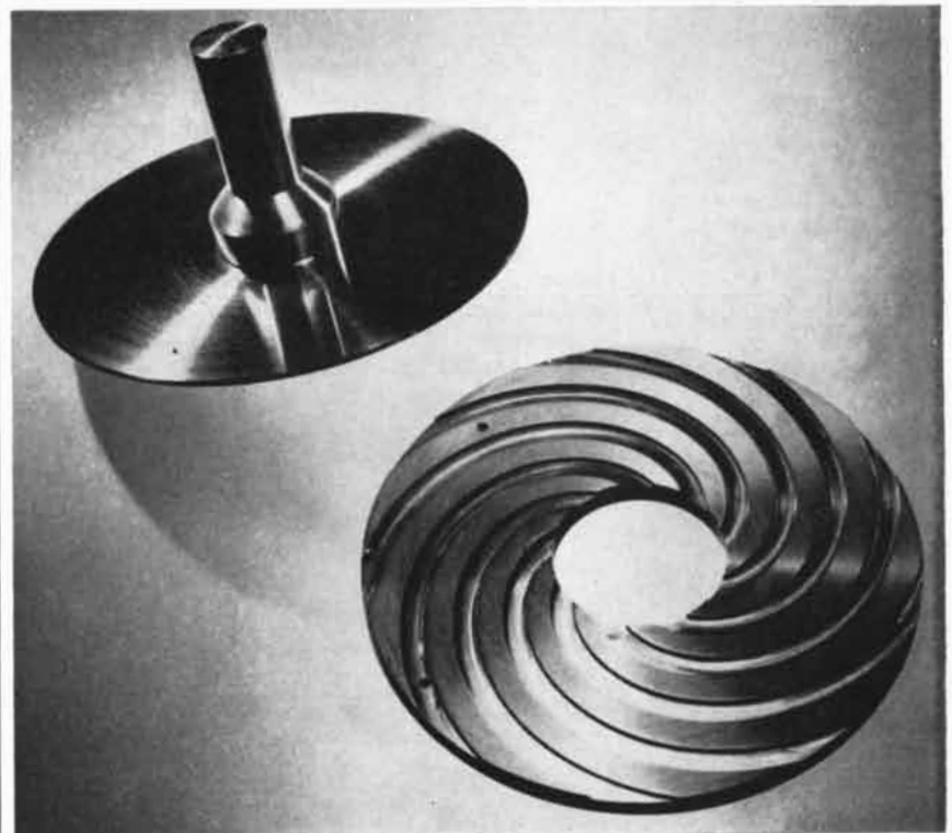
HIGH-SPEED CENTRIFUGAL VACUUM PUMP in top photograph achieves a vacuum so nearly perfect that no gauge can measure it. Stator and rotor of the pump appear in bottom photograph. Air molecules are whirled outward along rotor grooves, producing vacuum.
