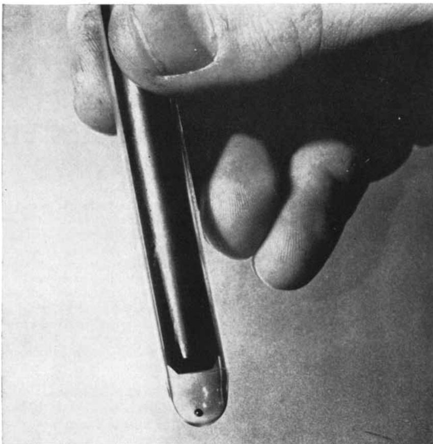
PELLET IN VACUUM TUBE , along with ferrite magnetic core, is inserted in apparatus shown on preceding page. There the tube is surrounded by liquid helium to increase vacuum.
