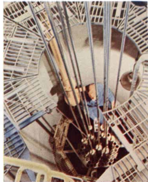
Critical Experiment Station. Low power test facility used to confirm physics of experiments before exposure in the reactor.
