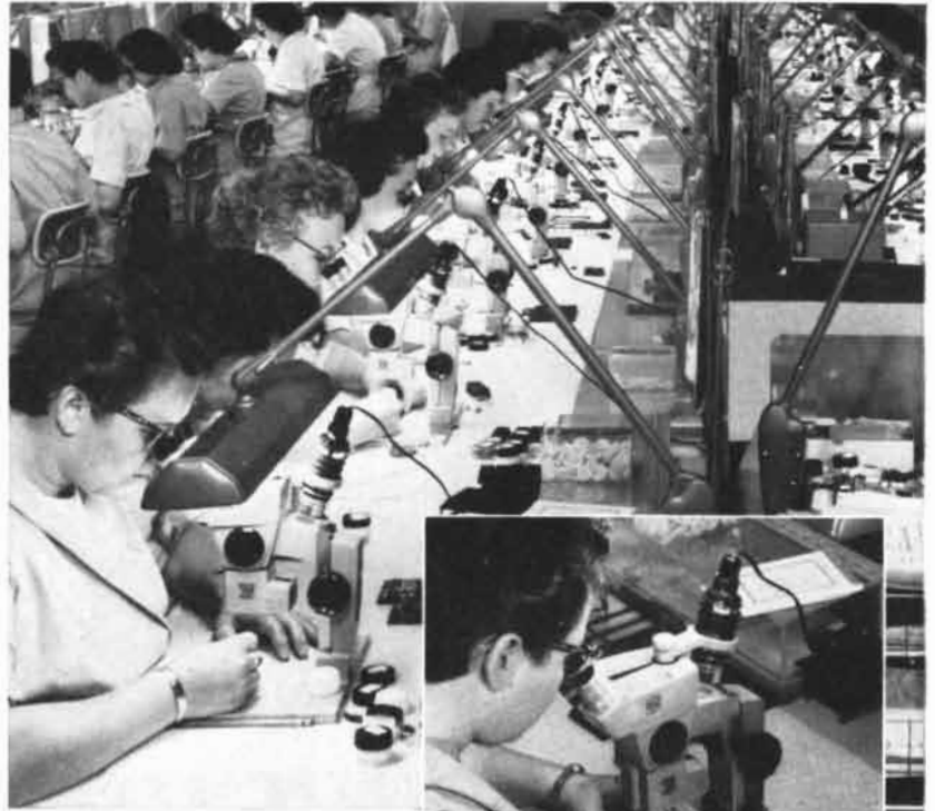
One of many assembly lines of skilled operators employing AO CYCLOPTIC Stereoscopic Microscopes to assemble advanced germanium computer transistors at Texas Instruments vast Semiconductor —Components division in Dallas, Texas.
