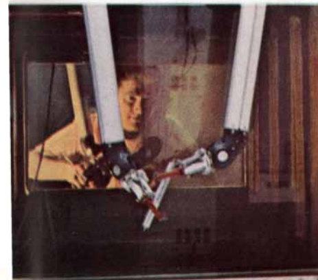
Remote Handling Facility. Hot cells and metallographic cells are available for post-irradiation examination of samples.
