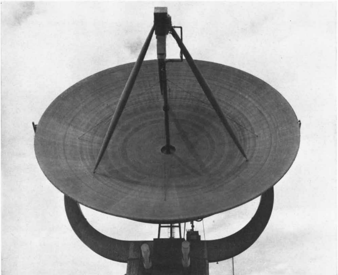
SOLID-STATE MASER is mounted at the focus of the 50-foot radio telescope as a preamplifier for the radiometer shown at top.
