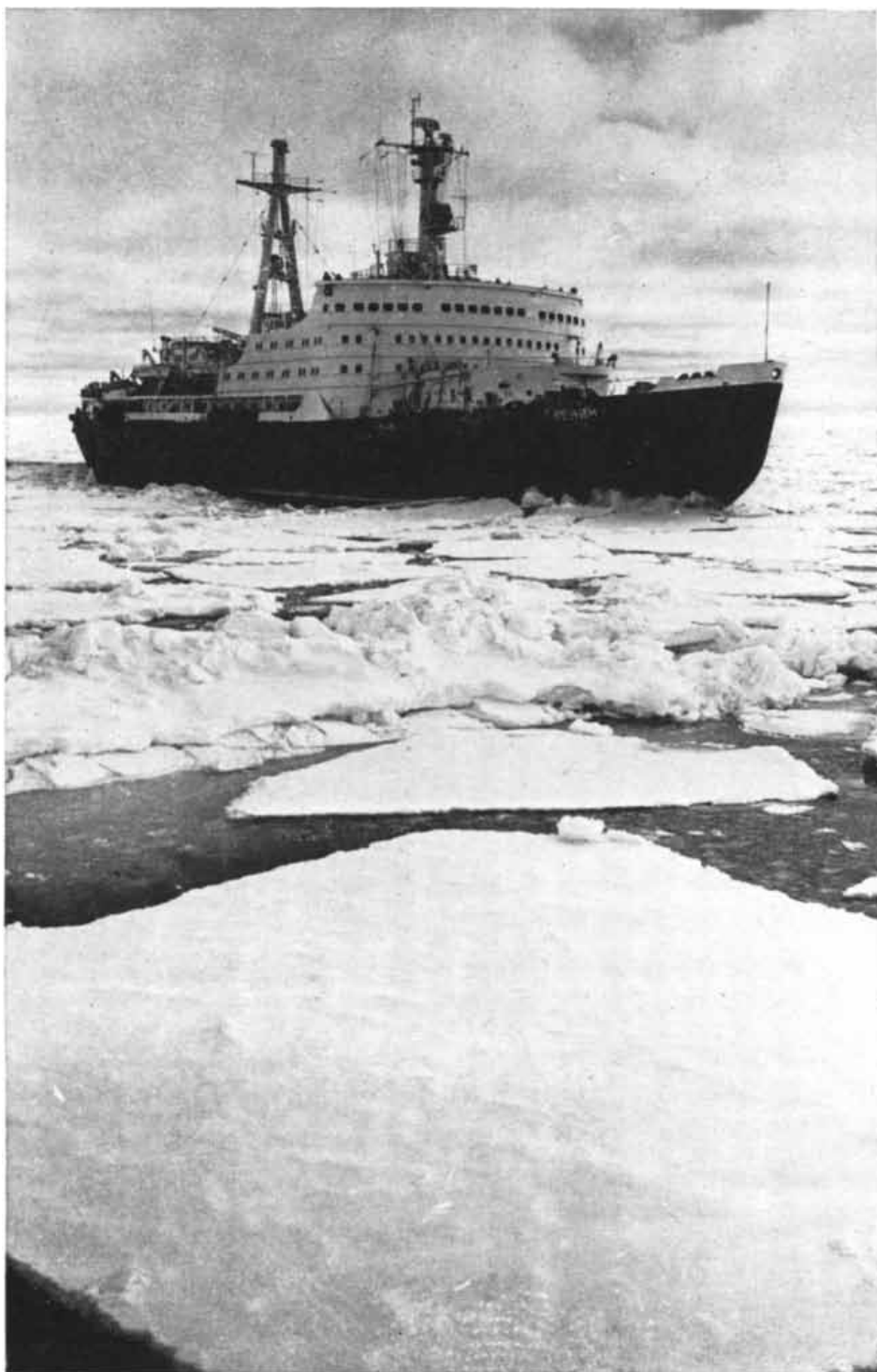
NUCLEAR-POWERED "LENIN" is late addition to Soviet fleet of icebreakers. Ships are used for scientific research and for clearing paths through ice for commercial vessels.
