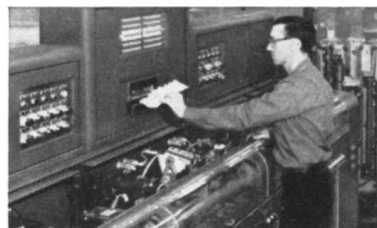
Contact verification machine, developed and built by Western Electric, being programmed to check wire blocks for dielectric breakdown, physical configuration, and palladium contacts.
