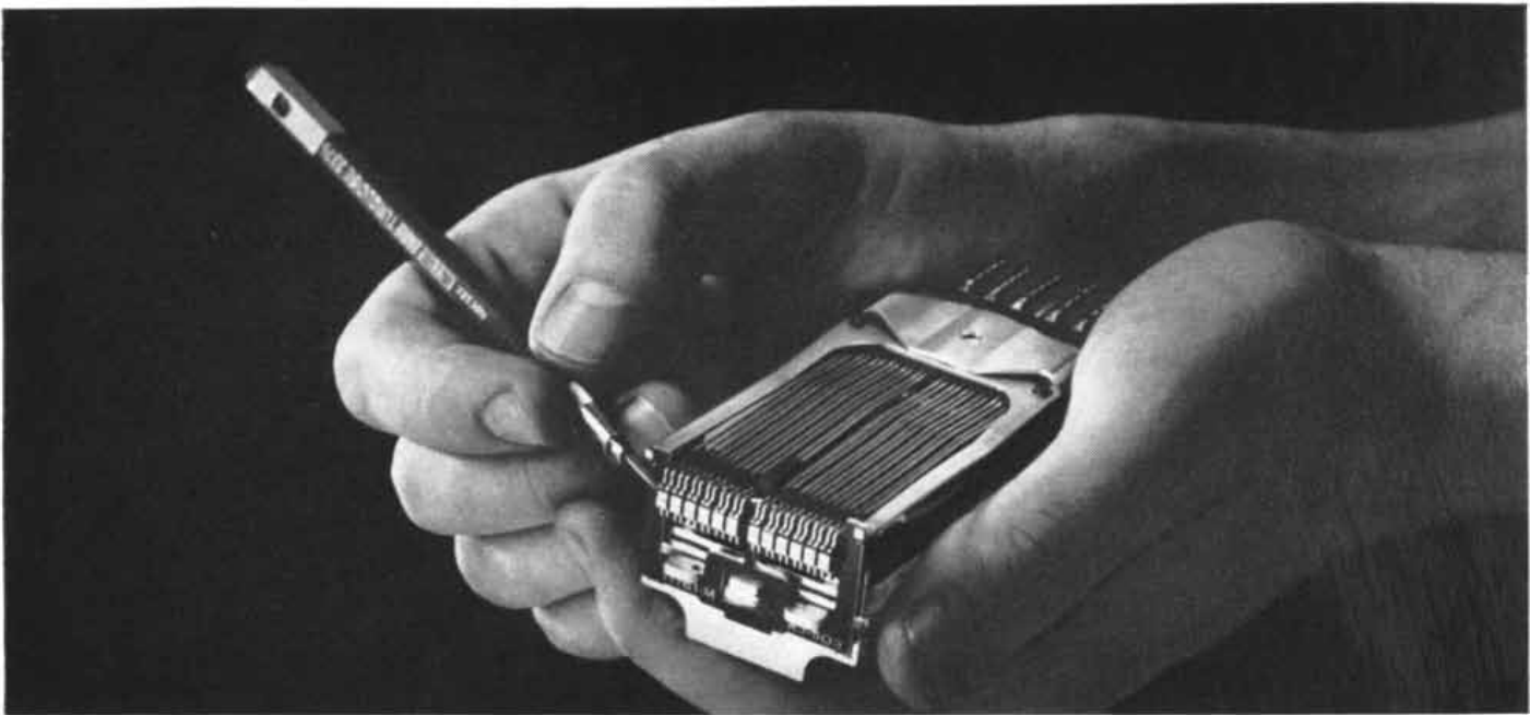
Hardly larger than cigarette packages, wire spring relays form the heart of switching apparatus for more than 200-million telephone calls a day. The pencil indicates the top row of tiny palladium-capped contacts which are vital to the relay's switching functions.
