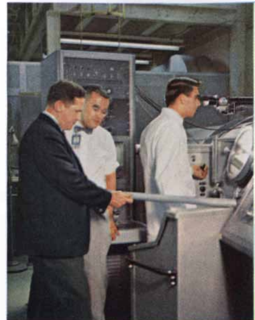
Electron Beam Welding of core components is one of the many special skills employed at the Atomic Fuel Department, Cheswick, Pa. Standard products of the department are reactor cores and their components.
