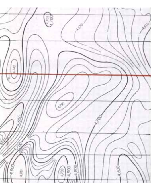
out on the map are identified. This one is for the flight line shown in red. Then the values indicated on the chart are transferred to the corresponding points on the map. The peaks and depressions of the record show up as magnetic "hills" and "valleys" on the map.
