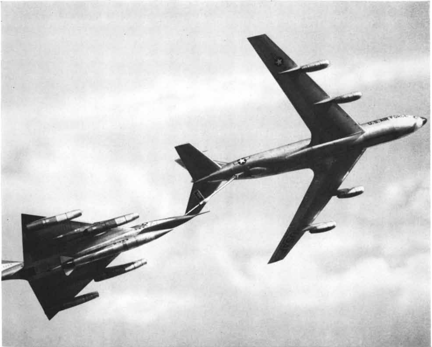
Bendix radar beacons enable B-58 (left), world's first supersonic bomber, to rendezvous day or night with KC-135 jet tanker. This aerial refueling makes it possible for the B-58 to reach any target in the world and return.
