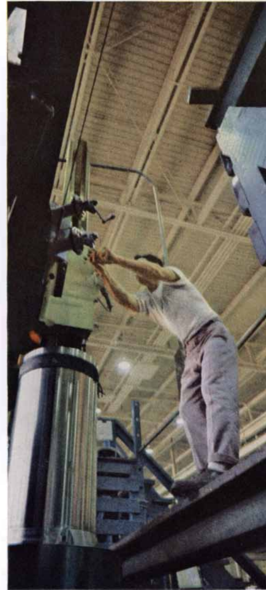
Skilled Machinist is working on the shell and flange for a canned motor pump on a 120" vertical boring mill at the Atomic Equipment Department.
