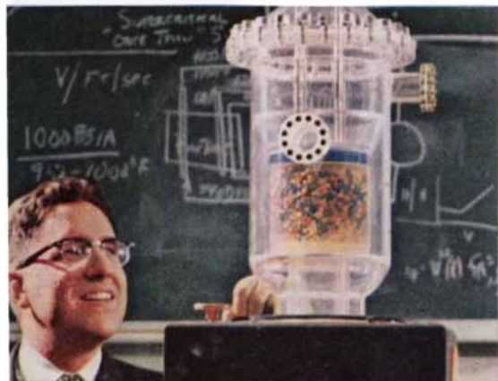
Dr. James H. Wright, shown here with an organic moderated fluidized bed reactor model, is also doing important development work on the concept of an integral boiling and superheat reactor (IBSHR).
