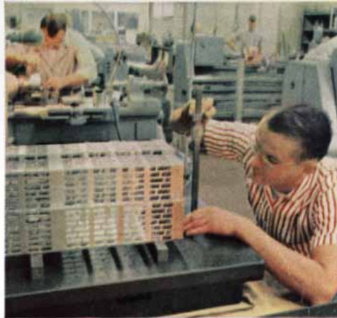
Fuel Assembly Operation at the Atomic Power Department, where facilities are maintained for development of advanced fuel concepts. Technician is working on cage of a fuel assembly.
