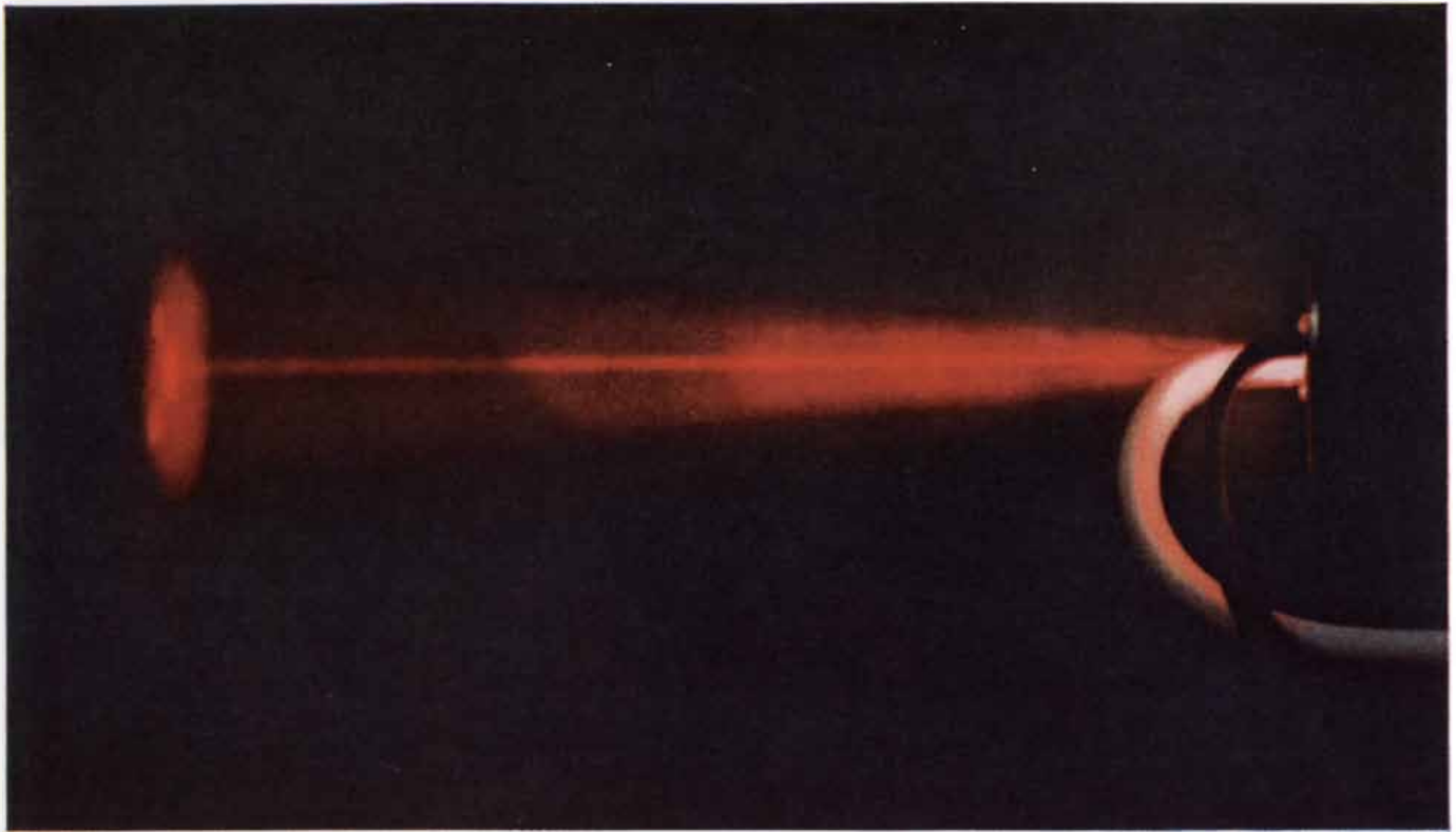
BEAM FROM RUBY OPTICAL MASER makes a thin streak of red light as it passes through smoke. Upper end of curved cooling
