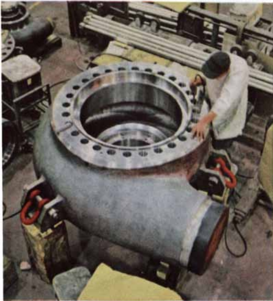
Westinghouse Quality Control inspector is working on a nine ton stainless steel pump casing at the Atomic Equipment Department in Cheswick, Pa. Department produces canned motor pumps, valves and control rod mechanisms.
