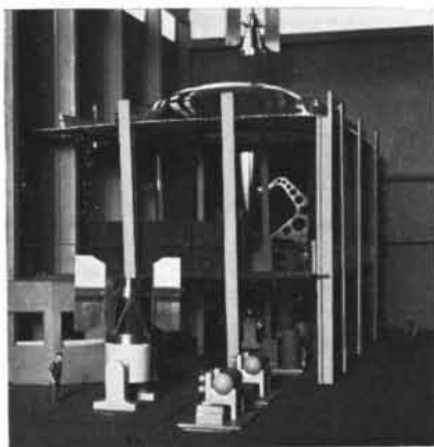
New Vibration System will include 28,000-pound exciter driven by an amplifier capable of delivering 140 KW over a frequency range of 25 to 10,000 cps.
