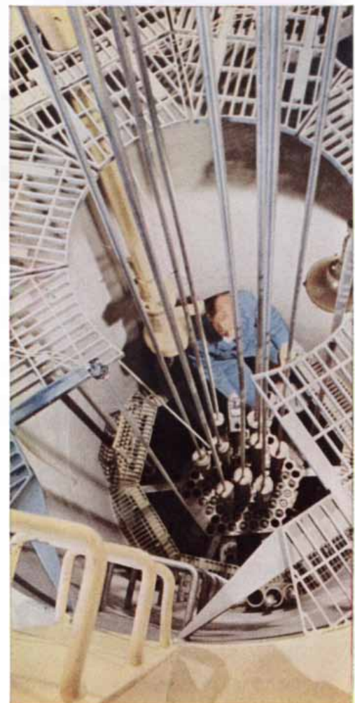
Critical Experiment Station at Testing Reactor. This technician is working in the low power test facility used to confirm physics calculations by experiments before exposure in the reactor.
