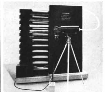
FEXITRON 201: 0.2 microsecond; 600 kv; 9 mm. source size; 64" high; penetrates 6" of aluminum; price $23,553.
