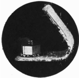
Example of metallic whisker growth on angle bracket
