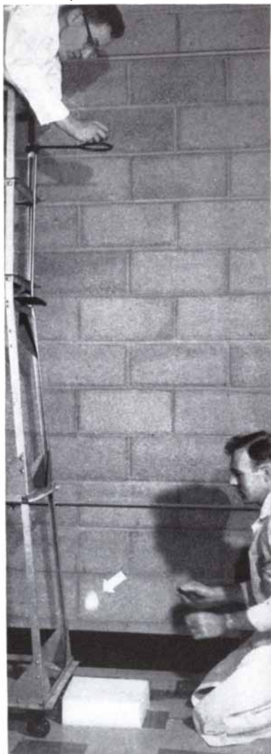
Egg bouncing from 12-foot drop shows cushioning properties of flexible urethane foam.
