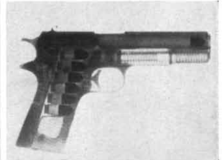
Ballistics: Radiograph of bullet at end of gun barrel; Fexitron 201 will expose film through 3" of steel.
