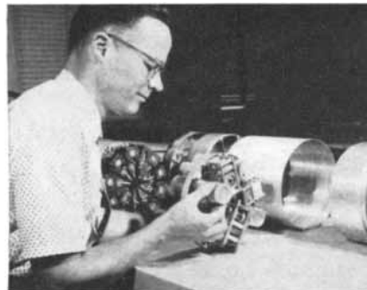
It was developing improved repeaters or “amplifiers” to increase greatly the capacity and economy of undersea telephone cable systems.
