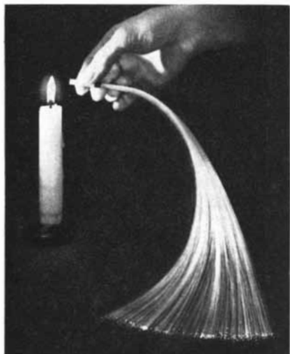
Candle demonstrates AO Fiber Optics in action. In a 50-micron fiber, a ray of light may be reflected 3,000 to 4,000 times per foot.
