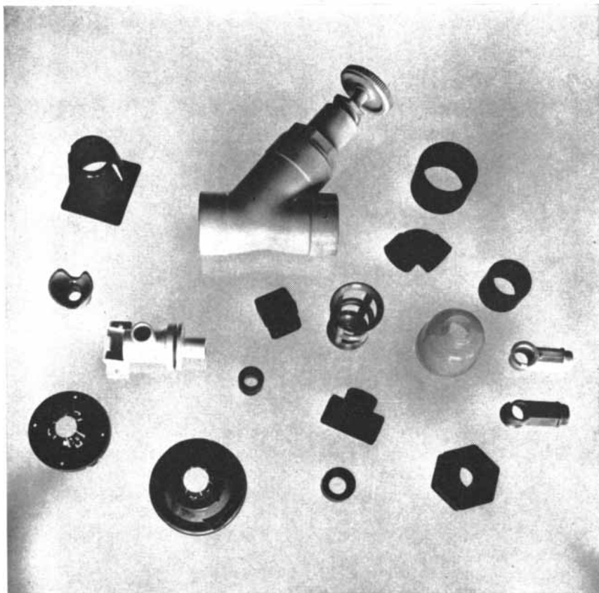
ARTICLES OF MOLDED POLYPROPYLENE yield tough parts and fittings coming into industrial use. In addition to strength the polymer has good heat and chemical resistance.
