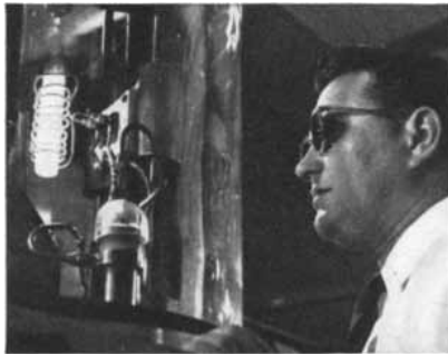
It was demonstrating the potentialities of the superconducting compound of niobium and tin for generating, with little power, magnetic fields of great strength.
