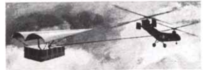
Ryan Flex Wing enables helicopters to tow several times the cargo or fuel they can carry
