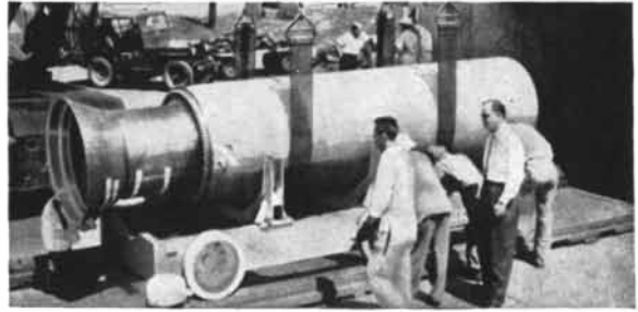
REDSTONE The most powerful single solid rocket booster ever fired in the free world—450,000 lbs. thrust—was developed for the Army's Nike Zeus program at Thiokol's Redstone Division. The motor is a product of research from propellant formation to scale-up and development of largest thrust rocket motor to-date.
