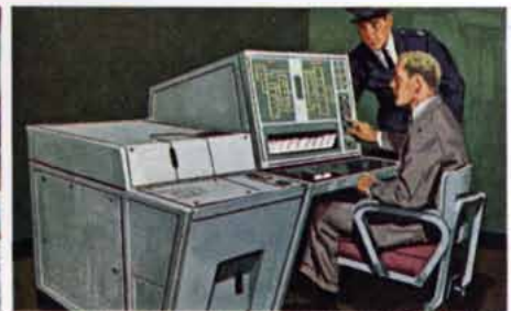
RCA's Automatic Checkout & Monitoring equipment continuously tests and checks performance of portions of the system and alerts an operator when a monitored signal exceeds certain limits.
