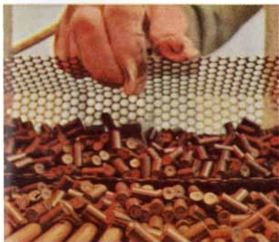
High Quality Pellets. Westinghouse can produce solid, hollow or spherical pellets, in sizes from .100" to approximately 1". A.F.D. has three compartmented pellet lines capable of simultaneously producing UO_2 pellets of three different enrichments.
