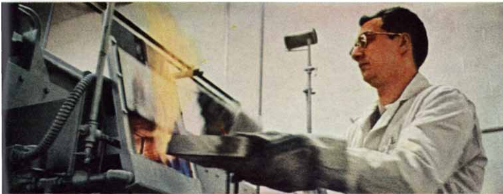
Modern Equipment. Facilities include pre-sintering and sintering furnaces (shown above), special vacuum welding boxes, vacuum annealing and vacuum induction melting furnaces, autoclaves for corrosion testing, rolling mills for hot and cold rolling, brazing equipment, brake presses for tube forming and plate bending. Other special production equipment includes a 48' high core assembly room with complete optical alignment and gaging equipment.
