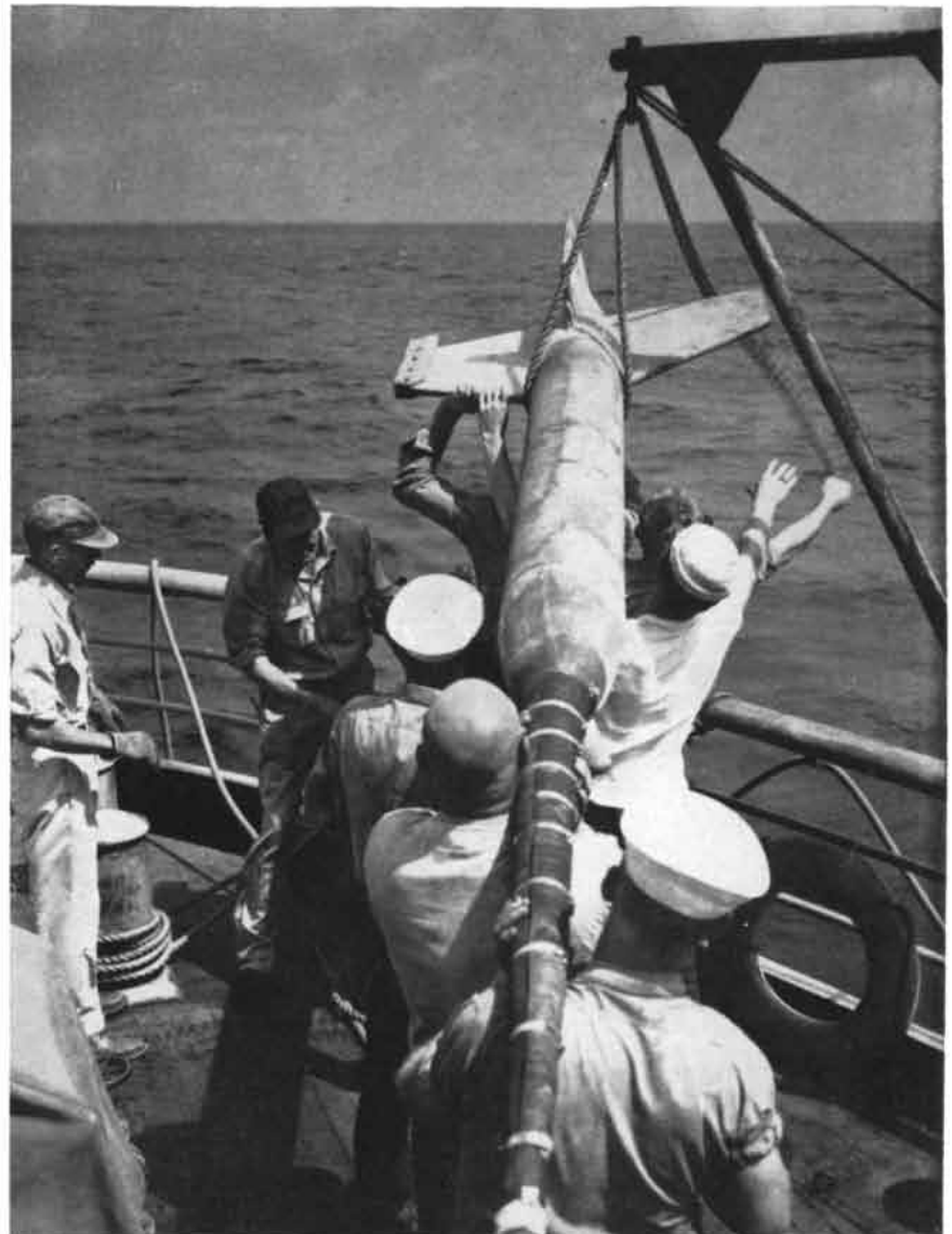
MAGNETOMETER IN ITS CASING is lowered into the water. It is towed at least 500 feet behind ship so that hull will not seriously distort geomagnetic-field measurements.
