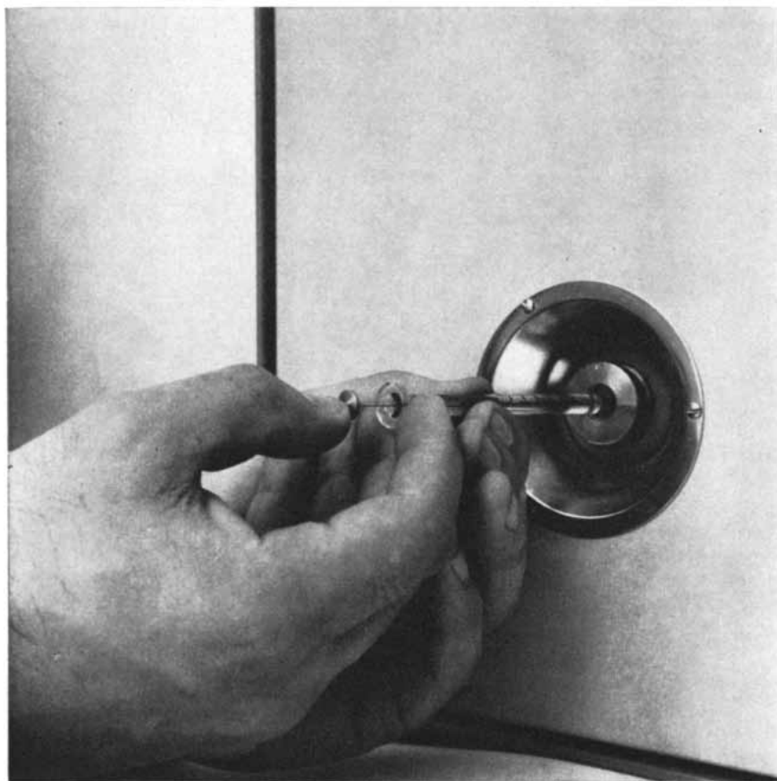
SAMPLE IS INJECTED into a gas chromatograph by means of a syringe that can deliver liquid samples as small as one hundred-thousandth of a cubic centimeter. Gas samples require a special valve arrangement to meter the sample through a chamber of known volume.
