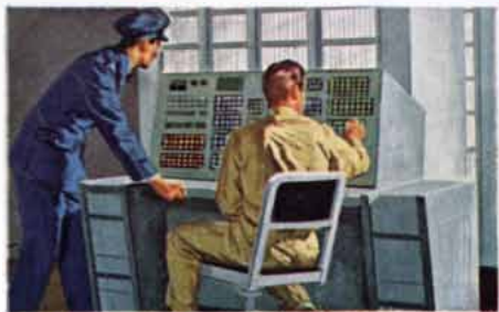
At NORAD Headquarters, RCA computing equipment, the Display Information Processor (control console shown here) receives sightings data from BMEWS and processes it for automatic readout.
