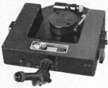
unisec measures angular precision of radar antennas
