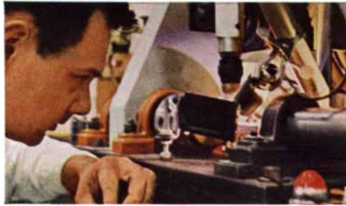
Rods and Assemblies. This technician is welding a stainless steel fuel rod. Westinghouse successfully fabricates aluminum, zircaloy and stainless steel rods and assemblies. Rods can be up to 1" in diameter and up to 130" long. Assemblies can be up to several thousand pounds.
