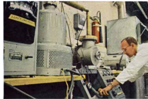
Fuel Development Laboratory. Each job is completely pre-engineered in a commercial fuel development laboratory. This engineer is sintering cermet in an experimental furnace with instrumented vacuum unit. Laboratory has equipment for development work on all types of potential fuel materials and processes.
