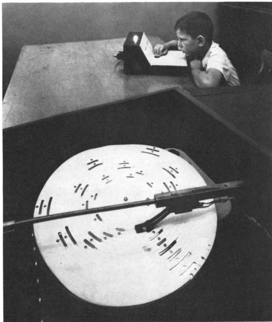
RHYTHM-TEACHING MACHINE requires a student to tap in unison with or echo a pattern of beats. To be reinforced by a light and a bell his response must fall within time limits set by a device ( foreground ) that both generates patterns and monitors responses.
