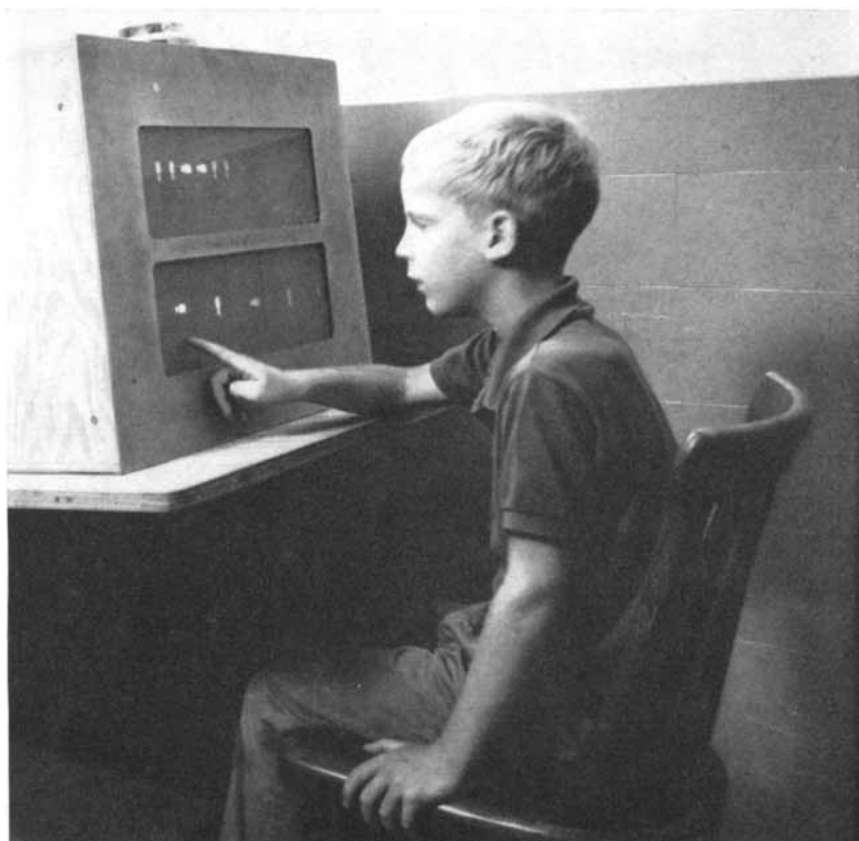
MACHINE FOR TEACHING INDUCTIVE REASONING presents a pattern at the top of a screen and below it a selection of responses on separate panels that are activated by touch. When the student responds correctly, he is “reinforced” (rewarded) by hearing a musical chime and seeing a light; part of his reward is seeing a new problem flash on the screen.
