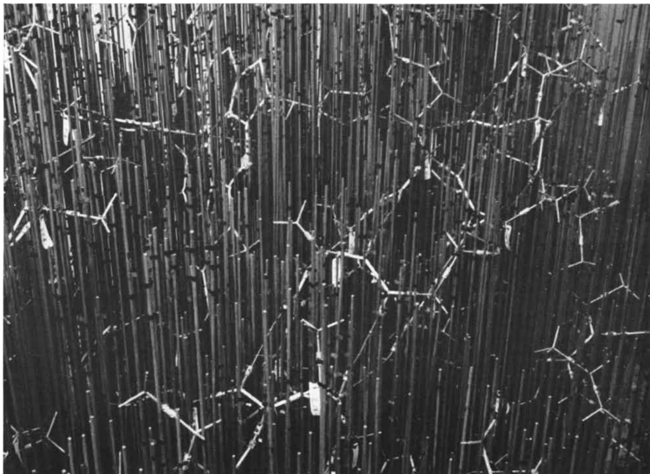
FOREST OF RODS was used to build up the two-angstrom model of the myoglobin molecule from electron-density map. Densities
