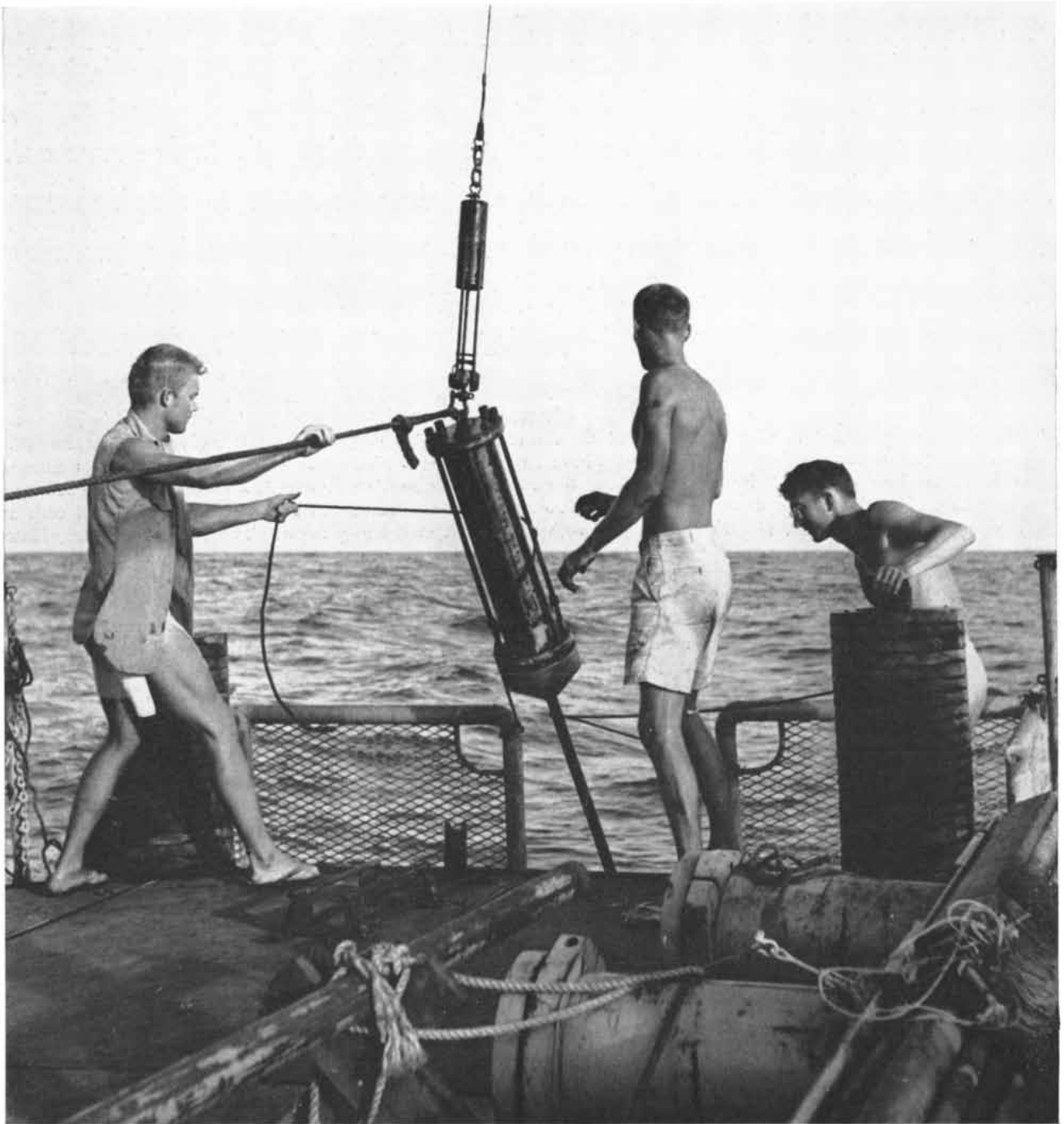
TEMPERATURE PROBE measures the heat flowing out of the earth's interior through the crust. The probe is the long slender tube. The watertight cylinder above it contains recording instruments. Here oceanographers are preparing to lower it into the water.
