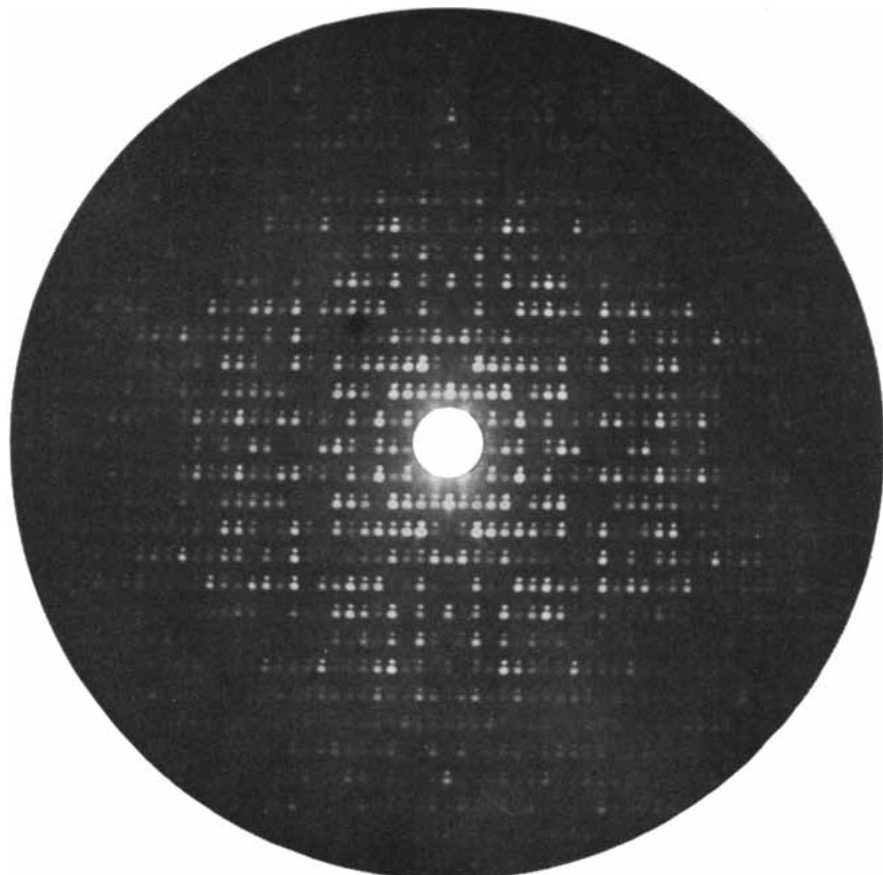
X-RAY PHOTOGRAPHS of myoglobin are patterns of spots. At top is a photograph of a normal crystal. At bottom is a photograph of a different type in which patterns of normal crystal and one labeled with heavy atoms are superimposed slightly out of register. Differences in density between two sets made it possible to determine phase of X-ray reflections.
