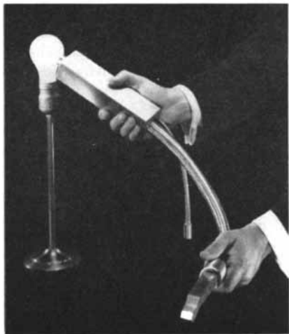
Illustration shows how fiber optics system transmits light along a flexible path. Shorter cable is light output monitoring device.
