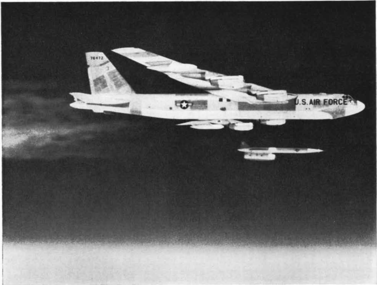
AERIAL MISSILE LAUNCHER. Photo shows Boeing B-52 missile bomber making in-flight launch of Hound Dog missile, which flies at supersonic speed toward target far ahead. In addition to missiles, versatile B-52s can carry regular bomb-bay load of
