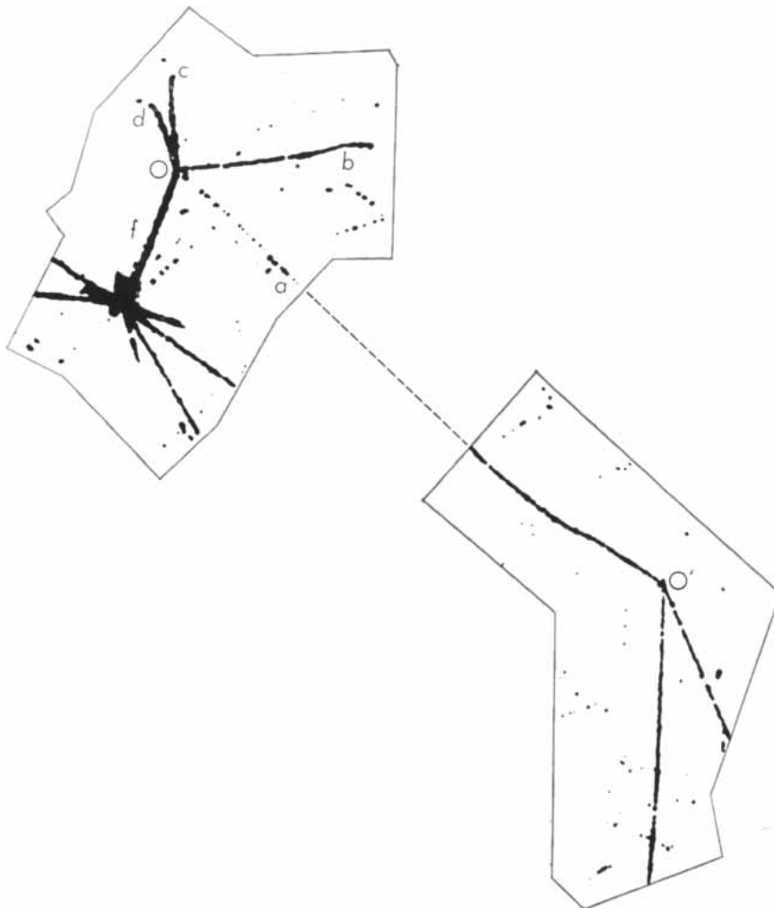
HYPERBERYLLIUM ( f ), resulting from the nuclear disintegration caused by a high-energy negative pi meson, decays mesonically "in flight" at O . The negative pi meson emitted ( a ) stops at O' and is captured by a nucleus, which it then disintegrates. Heavier particles (" b ," " c " and " d ") are emitted in a "forward" direction. The nuclear emulsion photomicrograph shown here in two sections was made by William E. Slater of the University of Chicago. The broken line is path taken by negative pi meson through emulsion.
