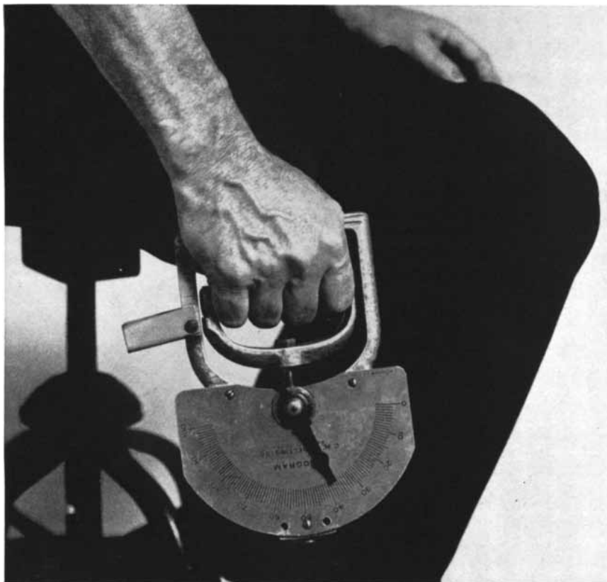
TEST OF GRIP STRENGTH serves to isolate muscle function. The subject squeezes the grip and the dial registers the amount of pressure, in kilograms, that he is able to exert.
