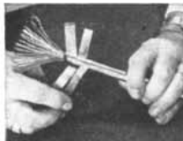
Shielding cables reduces magnetic radiation or pickup.
