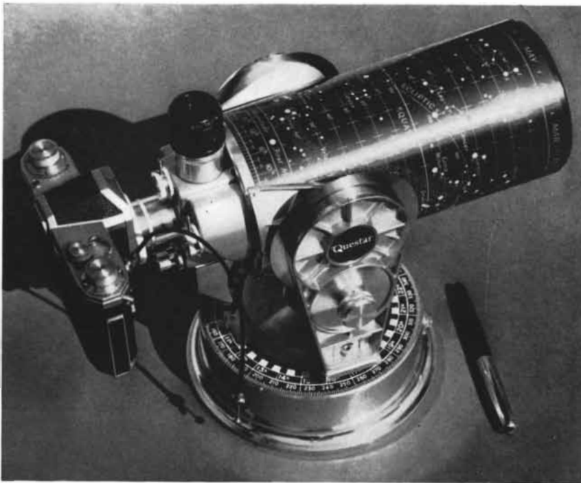
This is Questar with one of several suitable 35-mm. cameras attached. The telescope's 89-mm. aperture is always used wide open, since stopping down would only decrease the sharpness of this optical system. Only perfect optics resolve best at their full aperture.
