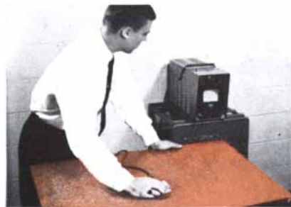
Preliminary ultrasonic test of copper plate for internal flaws; pickup crystal of test instrument is applied to each square inch of surface area. Subsequent tests involve up to 100% ultrasonic scanning of plate during total immersion in water.
