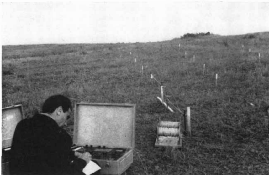
POTENTIOMETER is used to locate Etruscan tombs. At right are rows of electrodes stuck into the soil. Anomalies in readings from electrodes indicate presence of buried objects.
