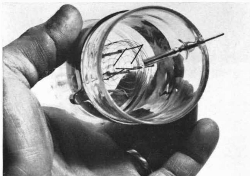
CONTROL PANEL (top) for pumps shown on page 79 includes a recorder (left) for ultrahigh vacuums and gauges (right) for earlier stages and subsidiary pumping systems. On the table in front is the Bayard-Alpert-type gauge to be installed in the chamber. In the close-up of the gauge (bottom) the transverse element is the ion collector, the fine spiral wire is the grid and the heavier diagonal wires are the filaments that supply electrons.
