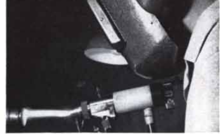
Extremely high temperature material problems encountered on re-entry into earth's atmosphere are studied with the aid of a plasma jet capable of 30,000°F.
