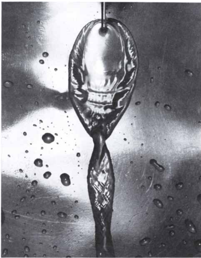
UNTREATED POLYETHYLENE SURFACE is not wetted by the jet of water seen in this flash photograph; the water is repelled.
