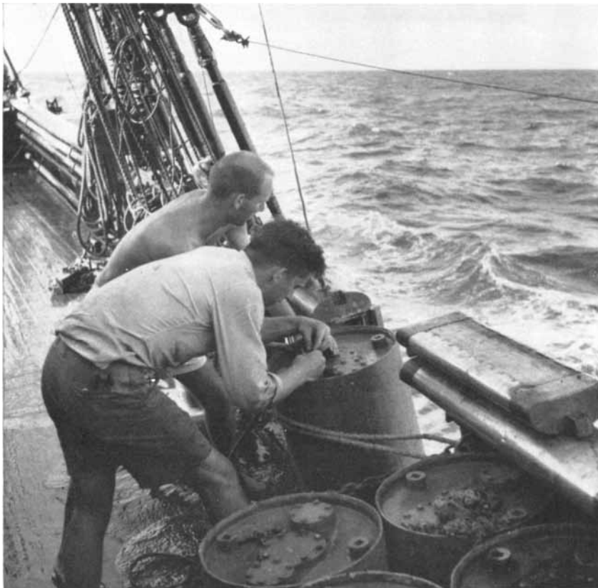
DEPTH CHARGE FUSE is lighted by Charles L. Drake as Maxwell stands by to help push the 300-pound charge through the rail of the Vema . These charges are used at relatively great distances from the listening ship; much smaller charges are used at closer distances.
