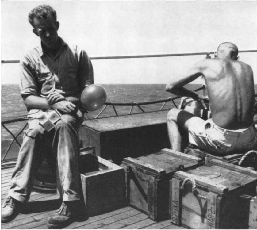
NINE-POUND FLOATED CHARGE is held by John E. Nafe (left), who will light the fuse and drop it overboard at a prearranged signal. In certain cases the gas bubble generated by an underwater shot gives rise to false reflection echoes; a charge kept afloat by a balloon, however, does not generate a gas bubble. At right Arthur E. Maxwell prepares another charge.
