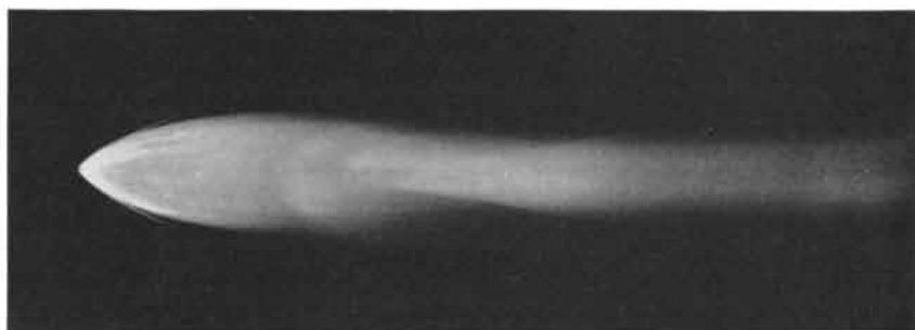
MIRROR BEHIND WIRE reflects light of explosion, showing head shock as luminous whiskers. Bright internal wedge is second shock wave expanding after it has converged.
