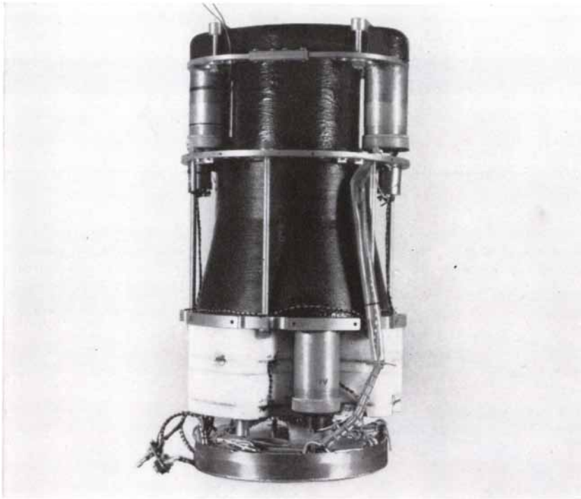
GAMMA RAY DETECTOR was designed and built in the Laboratory of Nuclear Science at the Massachusetts Institute of Technology. It weighs 30 pounds and is 20 inches high.
