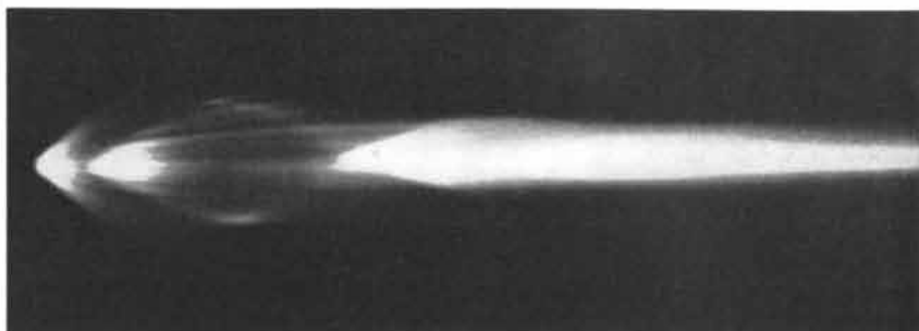
STREAK PICTURE lighted solely by wire itself shows peripheral arc ( tip ), which dies quickly, and internal arc, in which second shock converges, then expands ( bright wedge ).
