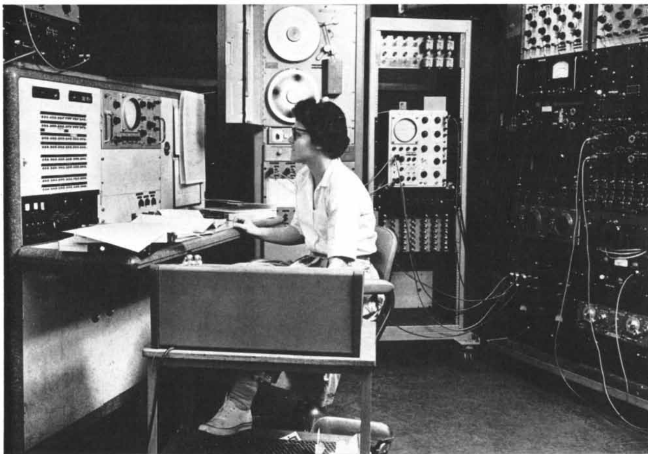
AVERAGE RESPONSE COMPUTER (ARC) was designed by W. A. Clark, Jr., of the Lincoln Laboratory of M.I.T. It samples the brain waves for a prescribed interval after each stimulus, adding and averaging the samples. Oscilloscope face on computer
