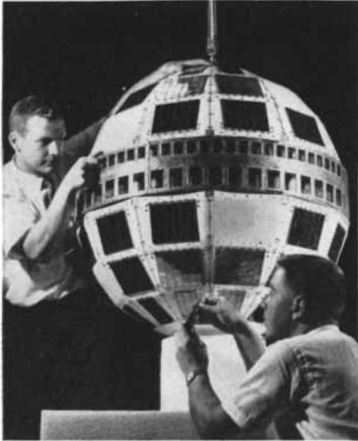
Telstar satellite —34" sphere has 72 gem-like facets, is intended for experiments in relaying telephone calls and other communications overseas. Solar cells convert sunlight into electricity. Launching is scheduled for this spring.
