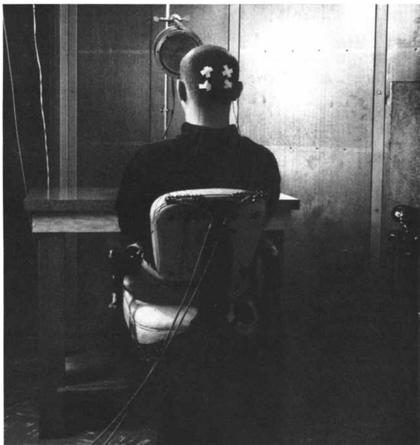
ELECTRODES ON SCALP detect brain waves. This subject, in an isolated room, is viewing brief flashes of light at regular intervals. A special computer simultaneously analyzes the brain waves from the visual region in back of head, producing the record seen in illustration on page 150. The photograph was made at the Massachusetts Institute of Technology.
