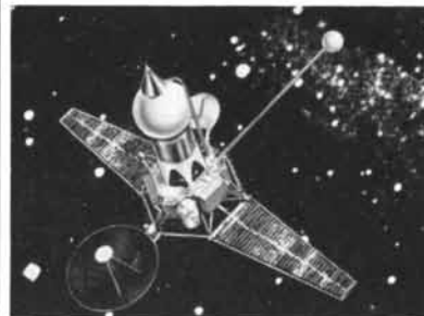
8,680 Hoffman Blue Space Cells produce 180 watts for Ranger lunar probe systems.
