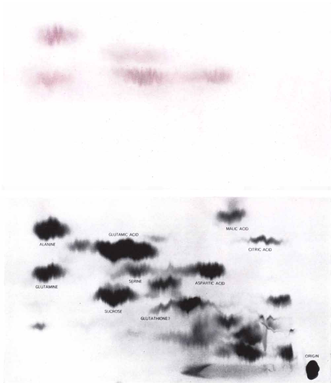
CHROMATOGRAM AND RADIOAUTOGRAPH used to corroborate the identity of amino acids produced by photosynthesizing algae appear at top and bottom respectively. The method of iden-
