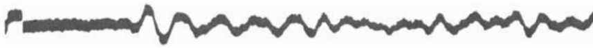
"LONESOME P" WAVE was recorded by Charles F. Richter and Beno Gutenberg of the California Institute of Technology, 8,000 kilometers from the Bikini "Baker" test of July 24, 1946. This trace covers less than one minute. The P wave is the only wave that appeared.
