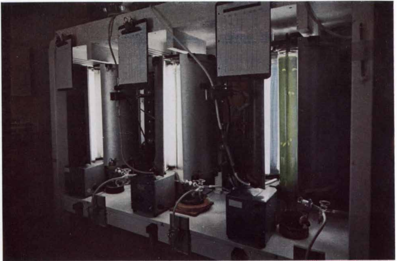
THREE CULTURE TUBES are part of the continuous-culture apparatus used by the Bio-Organic Chemistry Group at the University
