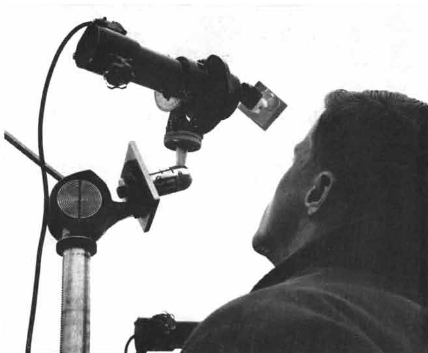
VIEWING ZENITH MOON , an observer looks up through the half-silvered mirror, which combines the reflected image of the infinitely distant moon with the background sky. In the actual experiment the subject places his eye almost directly against the glass plate.
