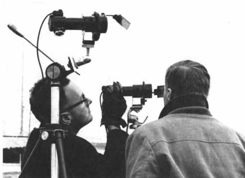
HORIZON MOON'S SIZE is adjusted by the experimenter until the observer says it is the same as that of the zenith moon. The ratio between the two sizes measures the illusion.
