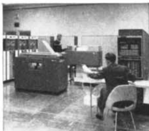
■ An IBM 1401 Data Processing System can be connected on-line to either of the two systems. Other data processing units can be added in building block fashion.
