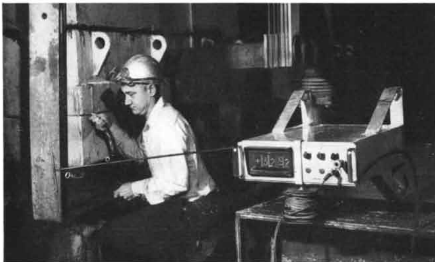
Digital voltmeter is used to detect small voltage drops.
