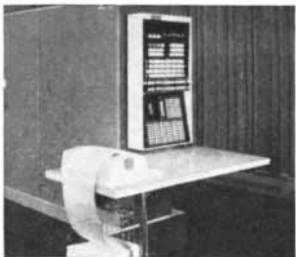
■ The new IBM 7040 Data Processing System for scientific computing, management science, and other data processing applications. Has a basic memory cycle of 8 microseconds.
