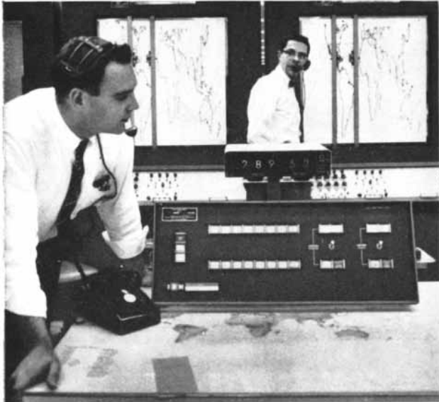
This plotting board, driven by an IBM computer, tells PROJECT MERCURY control personnel the exact location of the MERCURY spacecraft at any time in its orbit.
