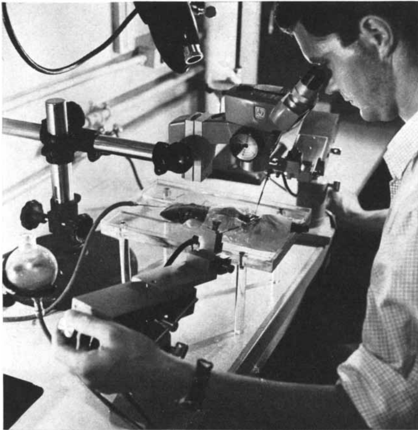
INSERTION OF MICROPIPETTE into a kidney tubule is accomplished with the aid of a pair of micromanipulators located at each side of a tray on which the anesthetized animal is placed ( center ). The experimenter monitors the operation through binocular microscope.
