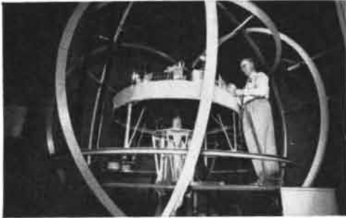
15 x 20-foot stainless steel Environmental Space Chamber simulates vacuumized conditions comparable to those found at 200 miles altitude.
