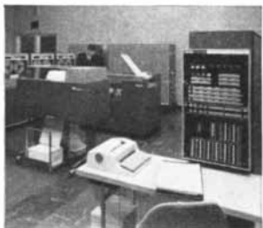
■ The 7044 Data Processing System has a 2.5 microsecond cycle. Both systems have memory capacities of 8,192, 16,384, and 32,768 words. The 7040 is available with a 4,096 word memory.
