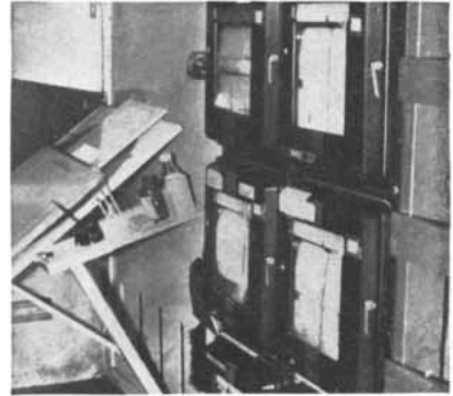
At this South Pole Station (and at the other four), sensors on the wind and temperature profile tower (above) detect ambient weather parameters. Speedomax G recorders (below) plot records of temperature and radiation.
