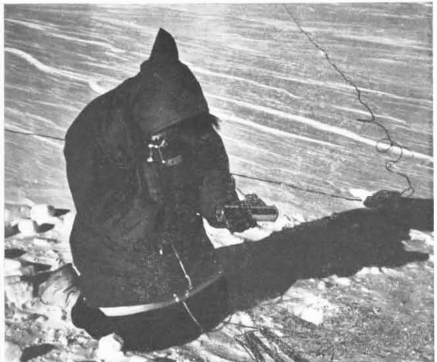
CHARGE IS SET for a seismic shot by Thomas Laudon of the Geophysical and Polar Research Center. Hole for charge is at lower right. Photograph was made by Behrendt.
