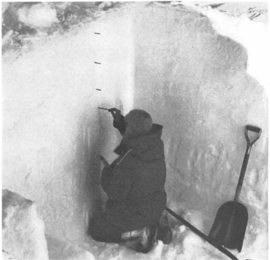
LAYERS OF SNOW are marked out with pencils by Gow at the beginning of a "pit study." The pit, which is about eight feet deep, is located near the snow mine at the South Pole.
