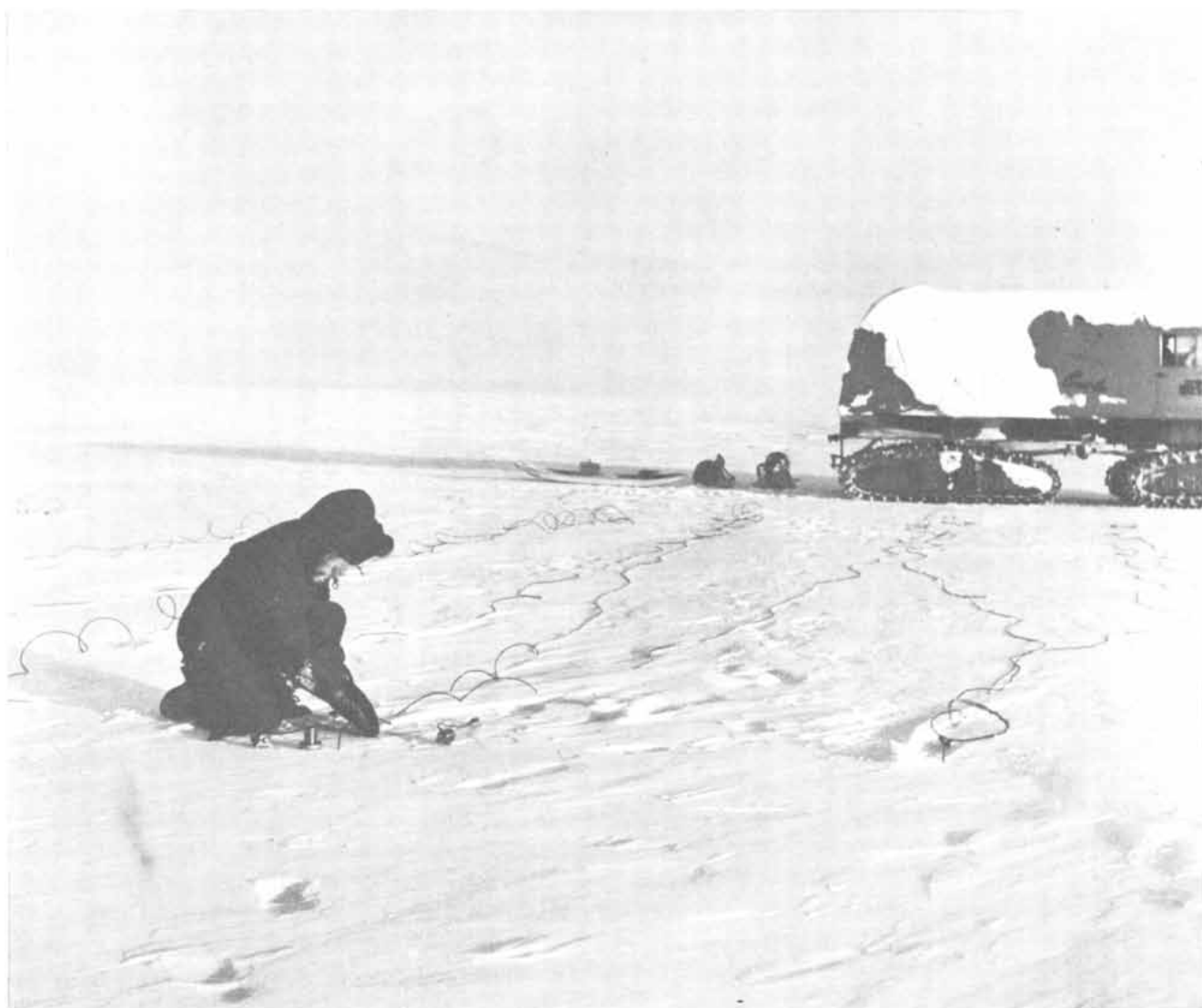
SEISMIC DISTURBANCES generated by explosive charges are detected by geophones, such as the one located on top of the snow
