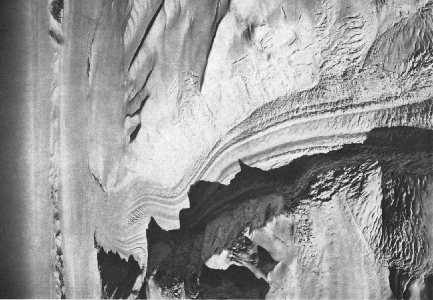
TRIMETROGON PHOTOGRAPH of Alice Glacier in Victoria Land was made from an altitude of 20,000 feet above sea level by a Navy photo-mapping aircraft. Sky is visible at far right and at
