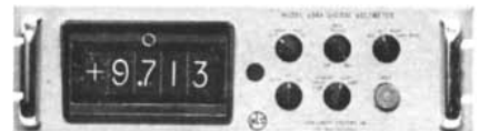
NLS V34A Digital Voltmeter. Five of these instruments are used in the Peoples system.
