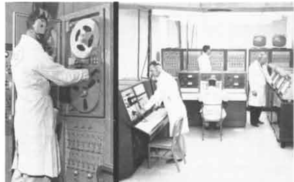
The Honeywell LAR 7400 FM tape system stores 14 channels of data
