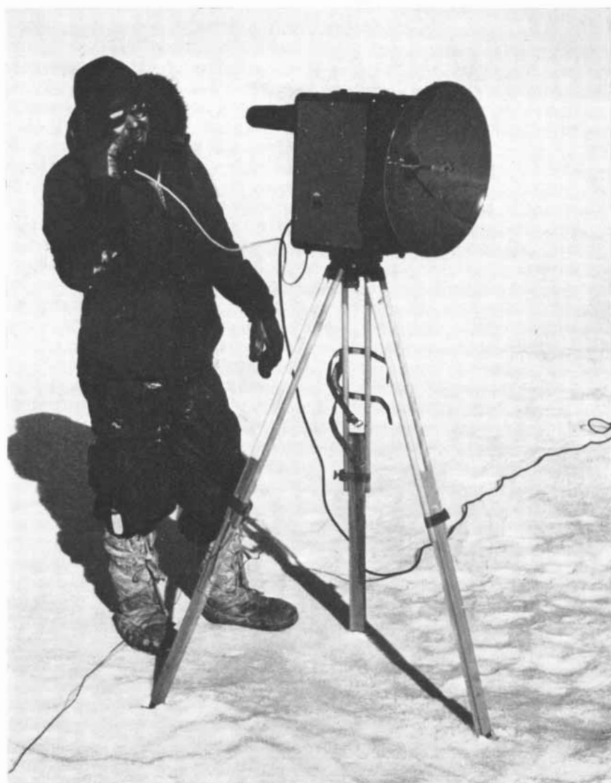
DISTANCE IS MEASURED between shot point and recording site with a tellurometer. Perry Parks of the Geophysical and Polar Research Center speaks to a colleague at the recording site. This photograph was made by John C. Behrendt, also a member of the Center.
