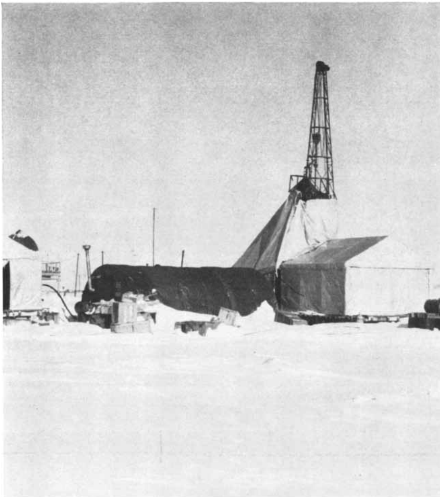
DEEP ICE-CORE DRILLING is done with this well-drilling rig at Little America on the Ross Ice Shelf. The drill derrick is 38 feet high. The photographs on these two pages were made by Anthony J. Gow of the U.S. Cold Regions Research and Engineering Laboratory.
