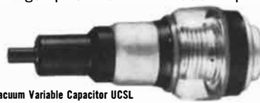
Vacuum Variable Capacitor UC5L 7 to 1000 mmfd Peak voltage—5 kv RF current—20 amps
