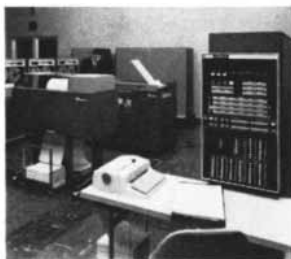
■ The 7044 Data Processing System has a 2.5 microsecond cycle. Both systems have memory capacities of 8,192, 16,384, and 32,768 words. The 7040 is available with a 4,096 word memory.
