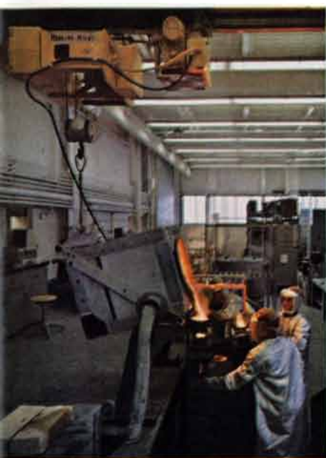
The A-L Processing Lab is equipped to melt by four different processes—air arc, air induction, vacuum arc and vacuum induction—and produces ingots from ½ to 500 lbs.
