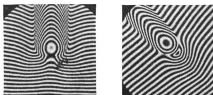
Ball track across copper crystal is narrower, harder and has higher friction in a cube diagonal direction (right interferogram) than in a cube edge direction.
