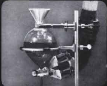
APPARATUS for studying the electric field generated by a bean root is shown in this photograph. The bean plant is held by a clamp at center. The glass tubes are probes to measure bioelectric potentials. The lens at left foreground projects a magnified image of the root.
