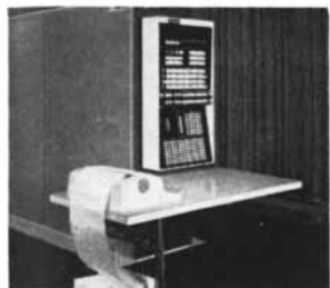
■ The new IBM 7040 Data Processing System for scientific computing, management science, and other data processing applications. It has a basic memory cycle of 8 microseconds.
