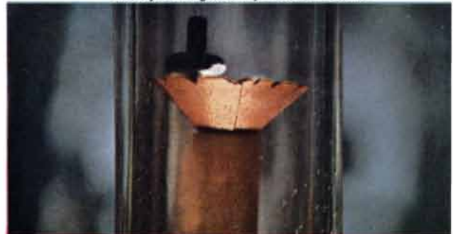
Analysis of gases by vacuum fusion.
