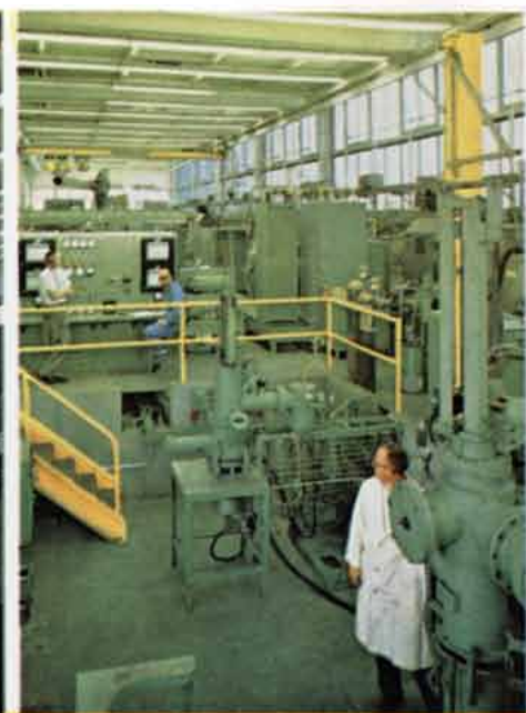
The A-L Processing Lab is equipped to melt by four different processes—air arc, air induction, vacuum arc and vacuum induction—and produces ingots from ½ to 500 lbs.
