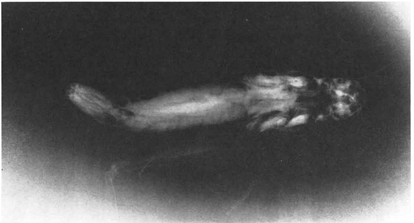
NEUTRON RADIOGRAPH OF GRASSHOPPER gives information that would be difficult to obtain in an X-ray picture. Tissue com-
