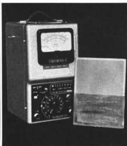
A copper conductive circuit board has been half-treated with UCAR 101 and then exposed to a sulphide atmosphere. While the unprotected half of the circuit board is greatly discolored, the treated portion retains its characteristic copper color.
