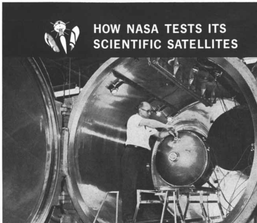
The 375-pound S-6 atmospheric measurement (135 to 540-mile altitude) satellite being readied to undergo space environmental testing in the Stokes-built and Stokes-designed Goddard "8 by 8."
